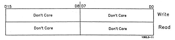
Any write to the SCSI utility register sets the initial DMA request for a SCSI data out transfer. This write must be done to initiate each new block. This write is done only after WDV is set in the control register, and just before DMA is set in the control register. Any read from the utility register will clear selected SCSI interrupts.
