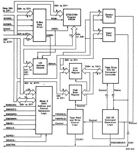
Figure 2-1. Quarter-Inch Cartridge Tape Module Functional Block Diagram
