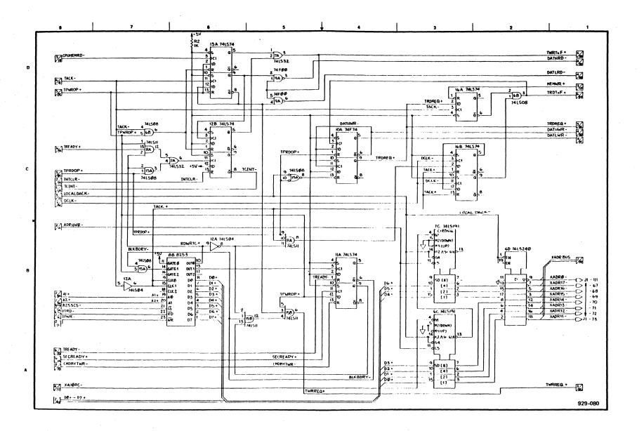
Figure B-1. Tape Control Board Schematic Diagram (Page 5 of 6)
