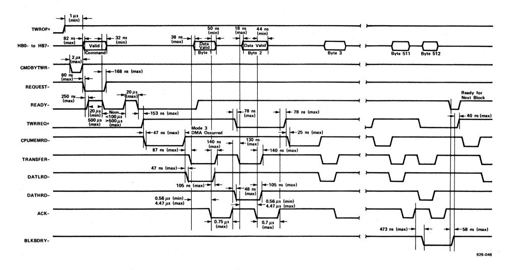
Figure 3-3. Write Tape Data Command Timing Diagram
