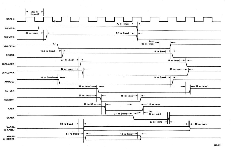
Figure 3-5. Mode 3 DMA Memory Write Timing Diagram
