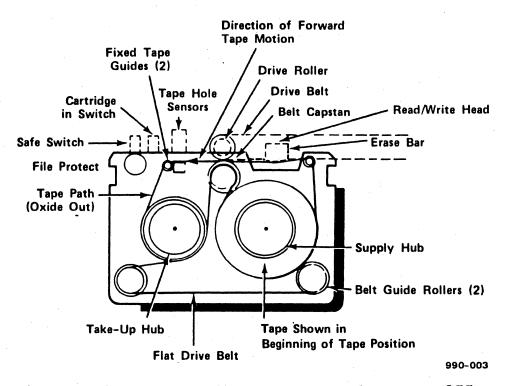
Figure C-1. Internal Components of the DC-600A Quarter-Inch Cartridge Tape
