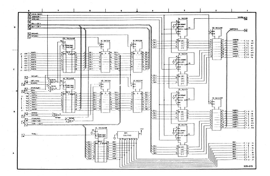
Figure B-1. Tape Control Board Schematic Diagram (Page 4 of 6)
