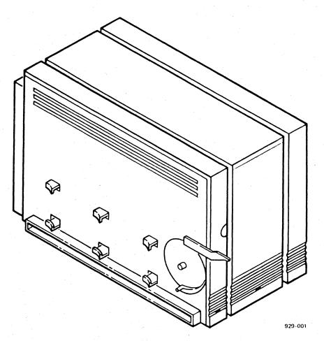
Figure 1-1. Quarter-Inch Cartridge Tape Module
