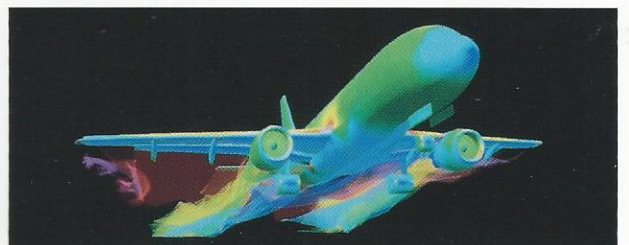
Right, airliner in ground effect. Image shows surface pressure distribution and wakes behind the aircraft.
