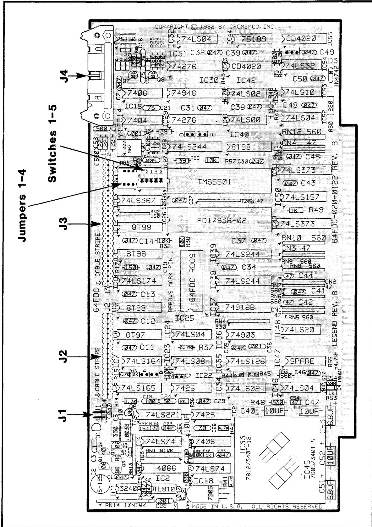
Figure 1-1: 64FDC SWITCHES, JUMPERS, AND CABLE CONNECTIONS
