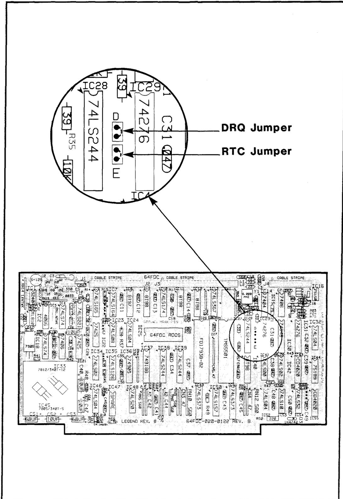
Figure 3-1: DRQ AND RTC JUMPER LOCATIONS
