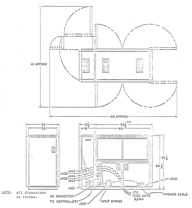
Figure 1, DIMENSIONS AND CABLING FOR THE BASIC 5022 SYSTEM.
