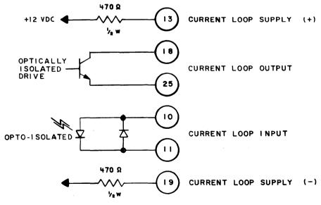
Figure 2-1 SCHEMATIC OF LINE JACK PIN ASSIGNMENTS
