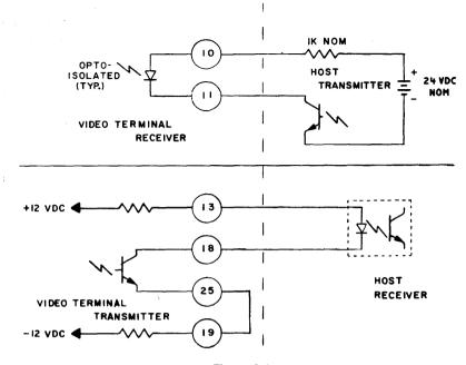
Figure 2-2 EXAMPLE OF LINE CONNECTOR USAGE
