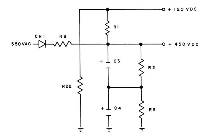
Figure 2-25. +120VDC and +450VDC Circuit
