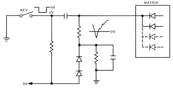
Figure 2-2. Typical Switch Circuit
