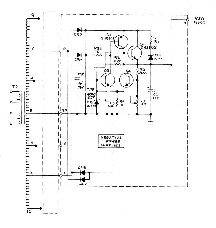
Figure 2-22. +13VDC Power Supply
