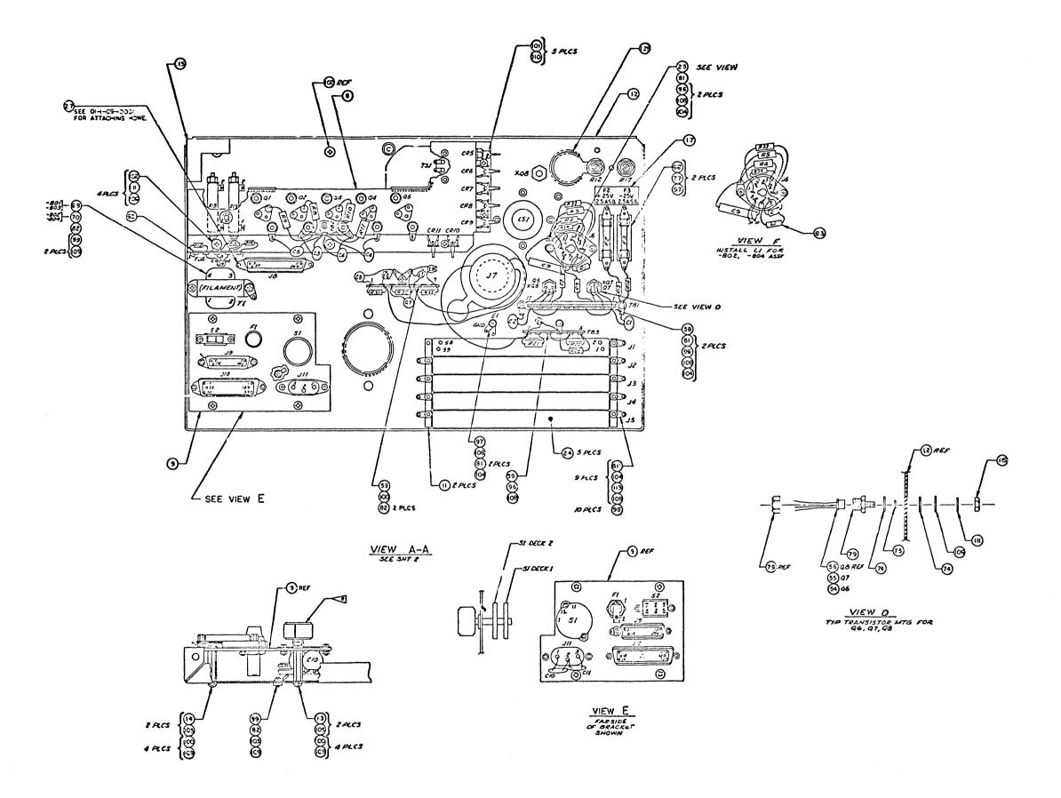
Figure 3-14. Rear Panel Assembly (2 of 3)
