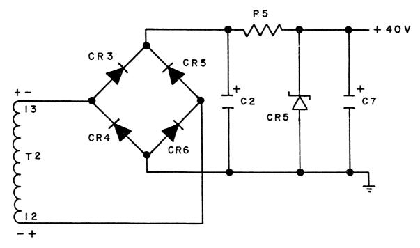
Figure 2-24. +40VDC Circuit
