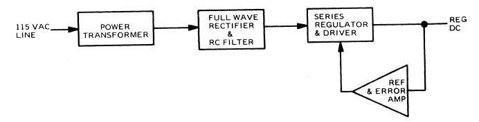
Figure 2-19. Typical Power Supply Block Diagram
