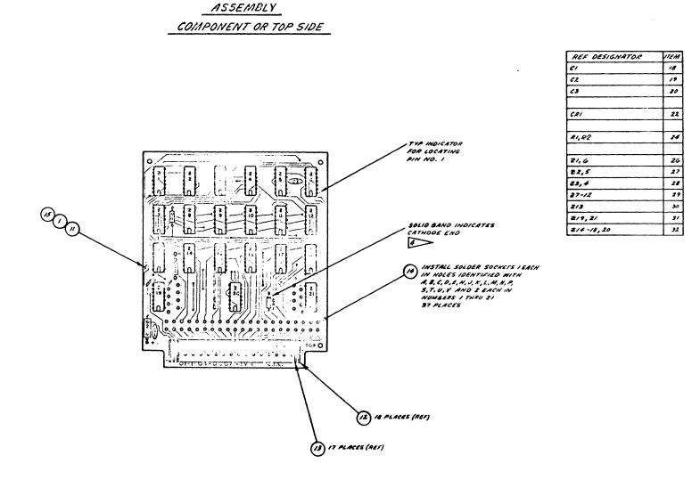
THE CATHODA END OF ALL DIODES IS INDICATED BY EITHER A COLOR BAND, A DOT, OR THE END FROM WHICH THE BANDS ORIGINATE.
