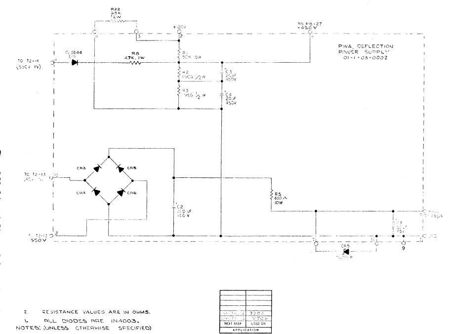
Figure 2-26. Schematic Diagram, Deflection Power Supply
