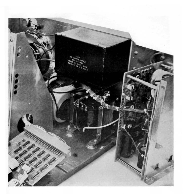
Figure 3-5. Logic and Deflection Power Supplies
