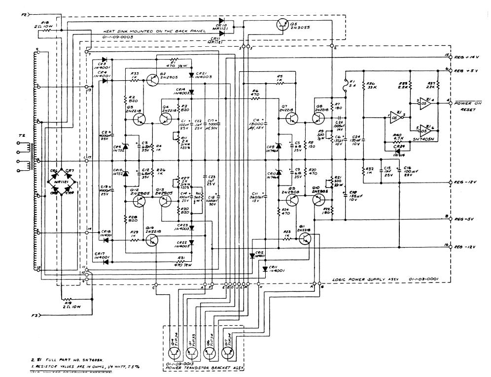
Figure 2-23. Schematic Diagram, Logic Power Supph 2-63/(2-64 blank
