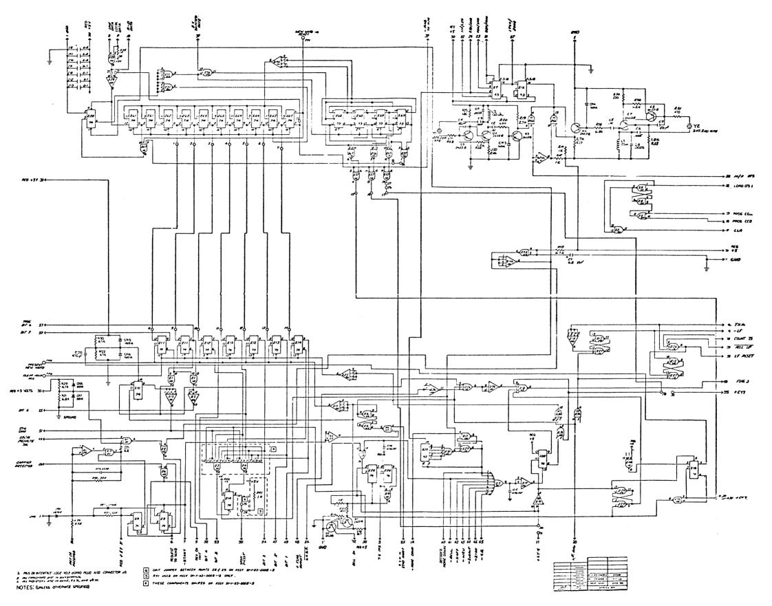
Figure 2-12. Schematic Diagram, Interface without Speed Buffer
