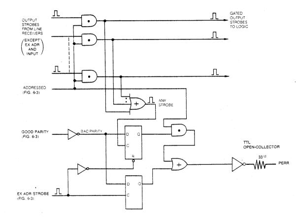
FIGURE 6-5 OUTPUT STROBE AND PARITY LOGIC
