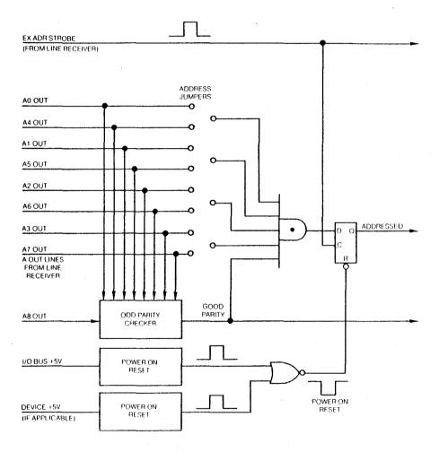
FIGURE 6-3 DEVICE ADDRESS LOGIC
