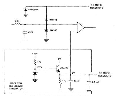
AQUT(-) RECEIVER (EXTERNAL DEVICES) FIGURE 6-1E
