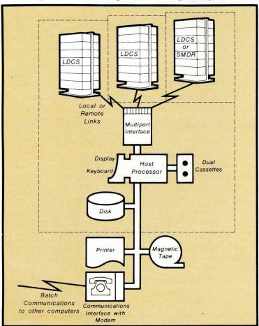
for long distance call control. The SMDR part is an intelligent metering subsystem for monitoring and collecting message details on all local calls, directory assistance calls, and tie-line calls processed by the system.
