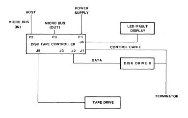
Disk expansion subsystem block diagram
