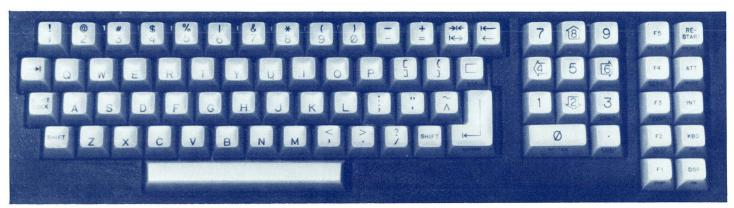
The photo above shows the Multipurpose keyboard with Word Processing/3270 option. Note the etchings on the front of the key caps.
