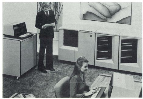
The new 9660 Laser Printer uses an electro-photographic printing unit to combine correspondence printing quality with high throughput. Its sophisticated paper handling capabilities offer routing to any selected output bin among as many as eight output modules.
