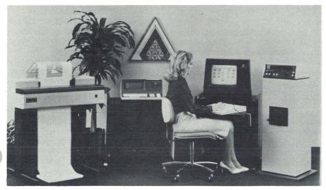
With the 9680 color graphics system ARC users can create color graphics images on a monitor screen with the help of an input stylus. Pictures can be output as hardcopy on a color dot matrix printer (left), as 35 mm slides or prints, or as 8x10 prints or transparencies (camera unit at right).
