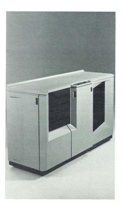
Datapoint's new 9660 Laser Printer is a laser-scanned electrophotographic, non-impact printer. The excellent print quality is one feature that makes the 9660 Laser Printer well suited for office applications.
