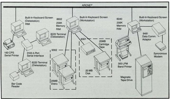
BUS applications. This workstation can also be used to run the DATAPOLL communications task by implementing the 9481 data communications adaptor attached to the 6040. It can also be used to drive a batch print job on the 300 LPM printer attached to the 6040, or to drive a batch print job on the 160 CPS printer.
