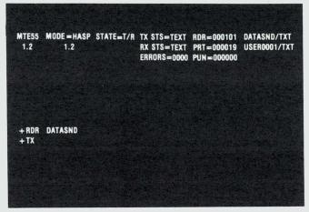
6000 Information Processing System. Teleprinter output can be directed to the console device. *MTERUP*
