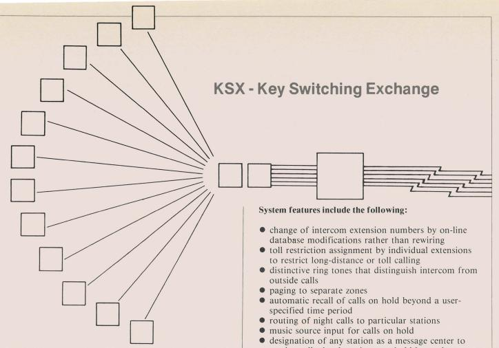
The Key Switching Exchange, KSX, is Datapoint's telephone system offering sophisticated features for handling the communications needs of a small business or branch office. Capable of handling from 8 to 128 phones, the KSX couples economy with growth potential.
