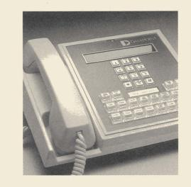
INFOSET II is the multi-line phone with 16 programmable keys for single-button line and feature selection. Selectable features include such things as automatic call back, call forwarding, call privacy, paging access, directed call pickup, leave message, and timed reminder. A built-in speaker gives you hands-free operation and a 24-character alphanumeric display presents status, call, or directory information.
