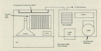
8600 Processor and 9301 Disk Drive: Internal Architecture
