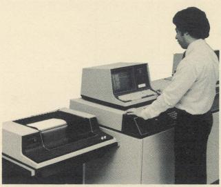
Manufacturing Systems' 8800 Processor with an 8200 Workstation as system console and 80 CPS printer for hard-copy output of system messages.
