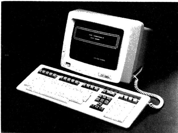
*The CIT-220+ is an ergonomically designed video terminal fully compatible with Digital's VT220, VT100 and VT52. The five programmable video attributes, multimode bidirectional auxiliary port and eleven setup menus enhance this unit's functional capabilities. The 12-inch diagonal, nonglare screen provides 24-line by 132/80-character column display.*
