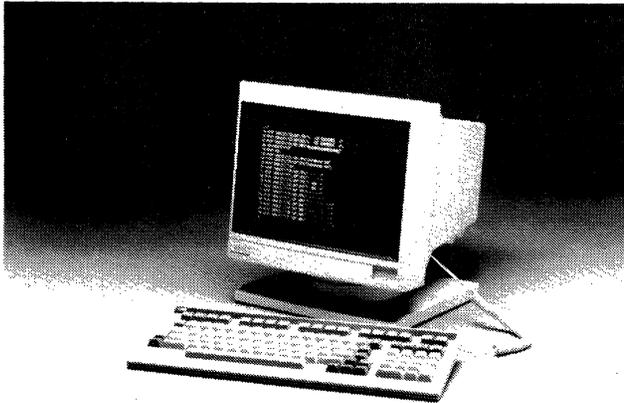
The ANT provides features normally found on other basic ASCII terminals. The unit contains a 14-inch nonglare amber screen with 24-line by 80 format and 25th status message line. It is fully compatible with the ADDS Viewpoint A2, IIT Qume QVT 101, TeleVideo 910, and Lear Siegler ADM 3A/5. The difference is the price—\$299. The ANT is currently the lowest priced alphanumeric terminal on the market.
