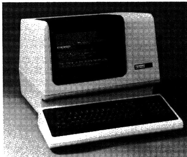
The DEC VT100 is one of the most popular, as well as one of the most widely emulated, video display terminals on the market today. When equipped with the Advanced Video Option, the terminal can display 24 lines of 80 or 132 characters, and features video attributes such as bold, blink, underline, and reverse on a character-by-character basis.
