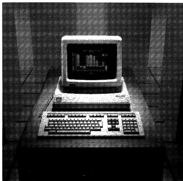
The VT240 is a monochrome terminal with both text and graphics display capability. Two graphics instruction sets are available for bit-mapped graphics displays. Screen resolution is 800 by 240 pixels.
