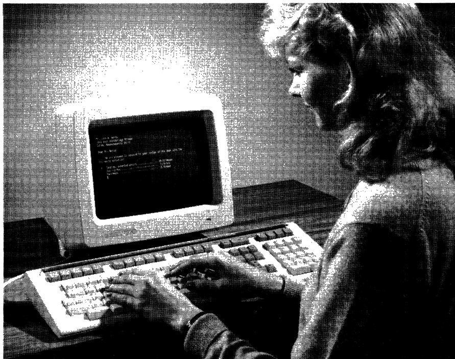
The Digital VT200 family of video display terminals consists of three models. The VT220 features full VT100 compatibility, the VT240 provides bit-mapped graphics architecture and text/graphics capabilities, and the VT241 replaces the monochrome display of the VT240 with a color monitor.
