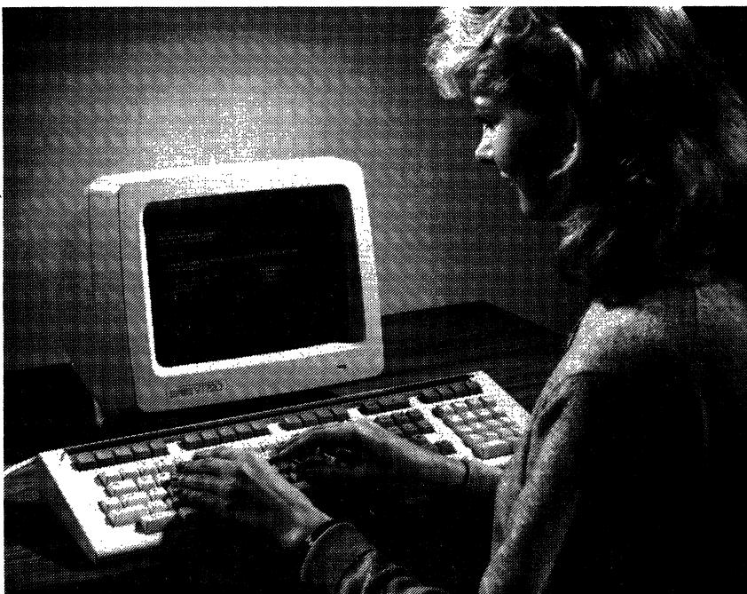
The Digital VT220 boasts full VT100 compatibility, including 80-/132-column display capability and compatibility with the ANSI X3.64 standard. As was the case with the VT100, several vendors have recently introduced terminals designed to emulate the VT220.
