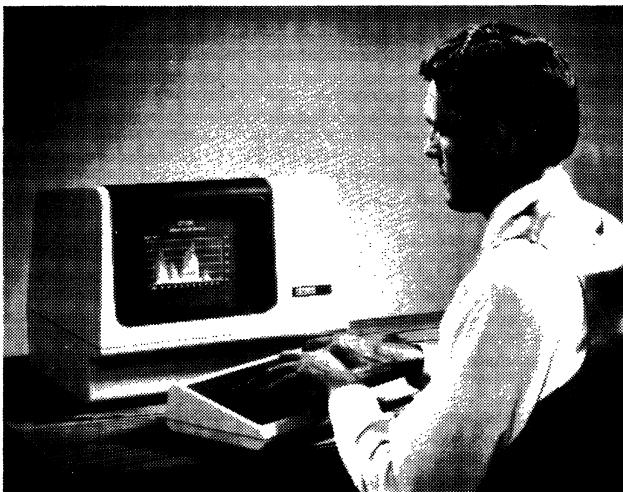
DEC's VT125 features business graphics, as well as alphanumeric, capabilities. Using DEC's Remote Graphics Instruction Set (ReGIS), pictorial data is created and stored as simple ASCII text. An upgrade kit is available to enable a standard VT100 to be configured with the graphics capabilities of the VT125.
