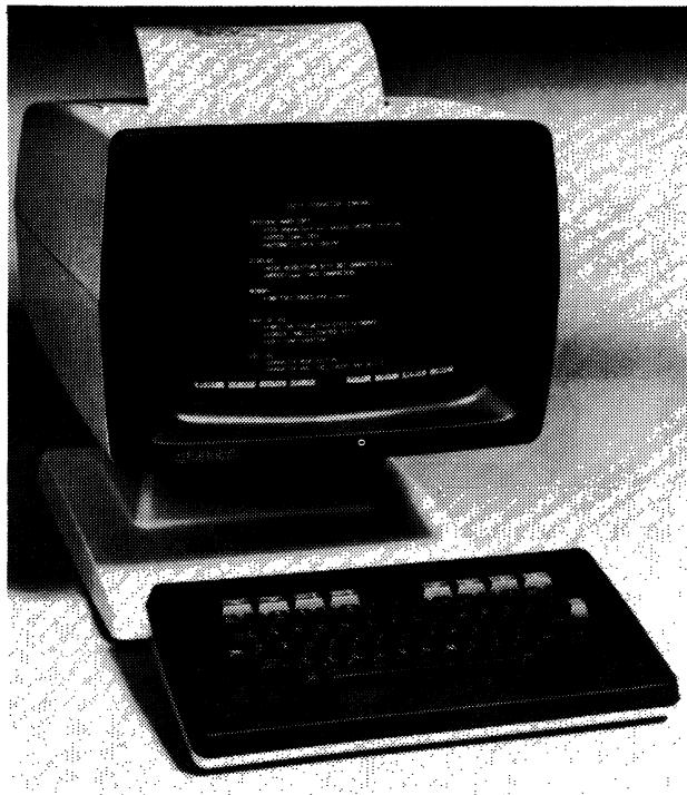
The HP 2621P has an integral thermal printer for hard copy output. Print speed is 120 characters per second.
