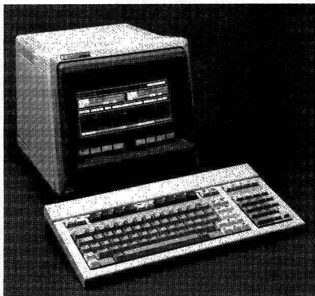
*The Hewlett-Packard HP 2392A is the company's newest display terminal. The HP 2392A features a new ergonomic design, including a compact 12-inch display (with integrated tilt/swivel mechanism) that takes up less desk space than previous H-P models. The detached keyboard features a new low-profile design and a two-position tilt adjustment. The HP 2392 also features Hewlett-Packard's lowest price ever for a display terminal—\$1,295.*
