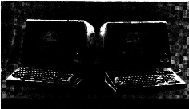
*The Executive 80 Series offers a variety of configurations and is designed for data entry, data inquiry, systems control, software development, and other applications.*
