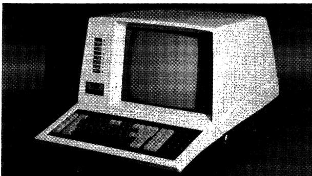
*The PTS-100 Display Terminal System consists of four controller models, offering support for up to 32 display stations, as well as a variety of other peripherals. The PTS-100 display, shown here, is available in 9-inch as well as 15-inch screen versions. Display capacities range from 480 to 1920 characters, with the following display arrangements: 12 lines by 40 characters; 15 lines by 64 characters; 12 lines by 80 characters; 24 lines by 80 characters; and 30 lines by 64 characters.*
