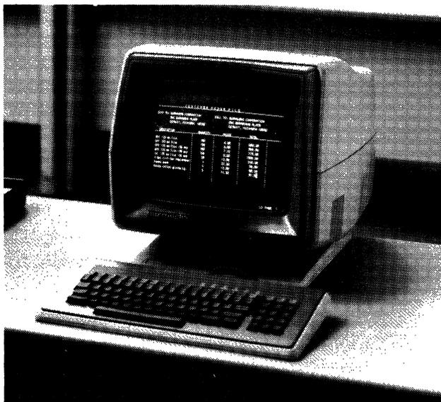
The ET 1100 display terminal is Unisys' general-purpose workstation for the company's computer systems. The standard ET 1100 is equipped with RS-232-C/TDI interfacing; the ET 1101 version features UDAA communications.
