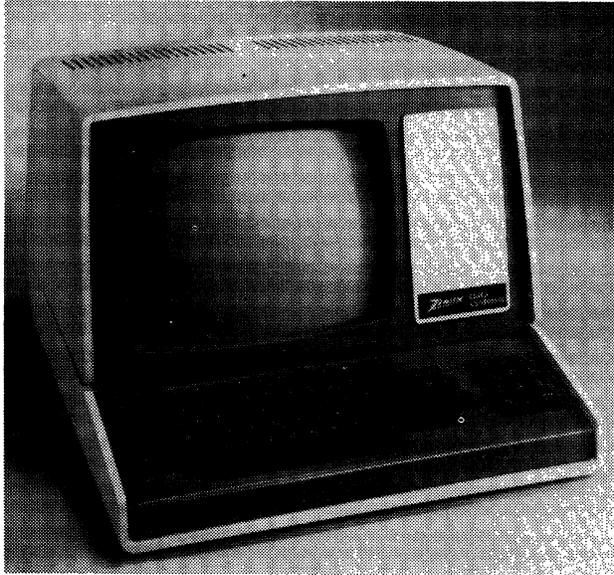
The Zenith Z19 Video Terminal features a 12-inch, non-glare screen with a capacity of 2000 characters. In addition to the conventional typewriter keyboard, 12-key numeric pad and eight special function keys are standard.
