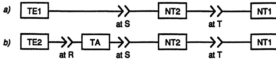
Configurations where ISDN physical interfaces occur at reference points S and T
