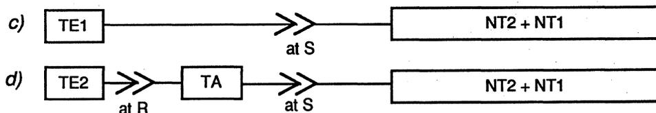
Configurations where ISDN physical interfaces occur at reference point S only
