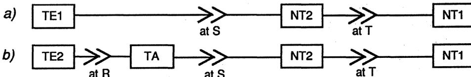
Configurations where ISDN physical interfaces occur at reference points S and T
