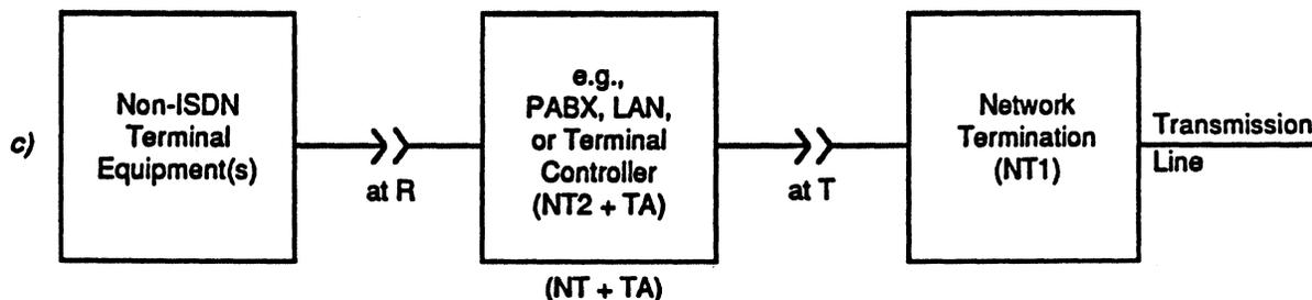
An implementation (see Figure 3f) where ISDN physical interfaces occur at reference point T but not S.
