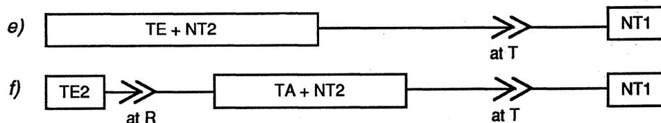
Configurations where ISDN physical interfaces occur at reference point T only
