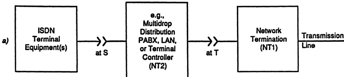
An implementation (see Figure 3a) where ISDN physical interfaces occur at reference points S and T.
