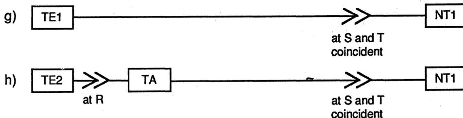
Configurations where a single ISDN physical interface occurs at a location where both reference points S and T coincide
