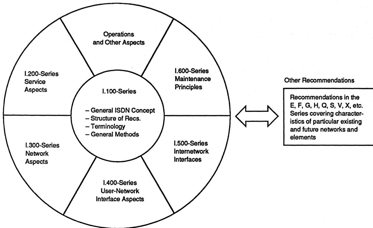
Note: Models, reference configurations, tools, methods, are contained in the appropriate I-Series Recommendations.
