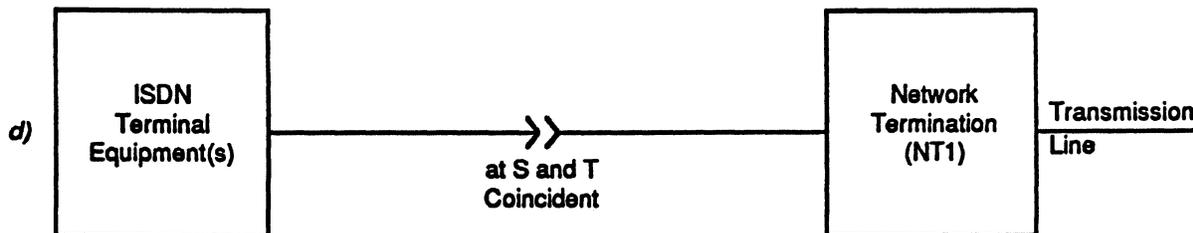
An implementation (see Figure 3g) where a single ISDN physical interface occurs at a location where both reference points S and T coincide.
