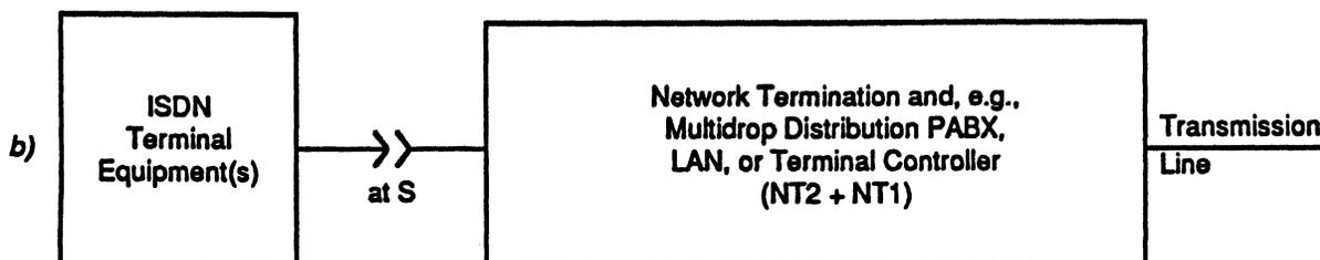
An implementation (see Figure 3c) where ISDN physical interfaces occur at reference point S but not T.
