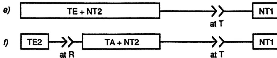
Configurations where ISDN physical interfaces occur at reference point T only
