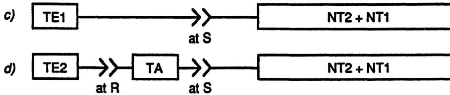
Configurations where ISDN physical interfaces occur at reference point S only
