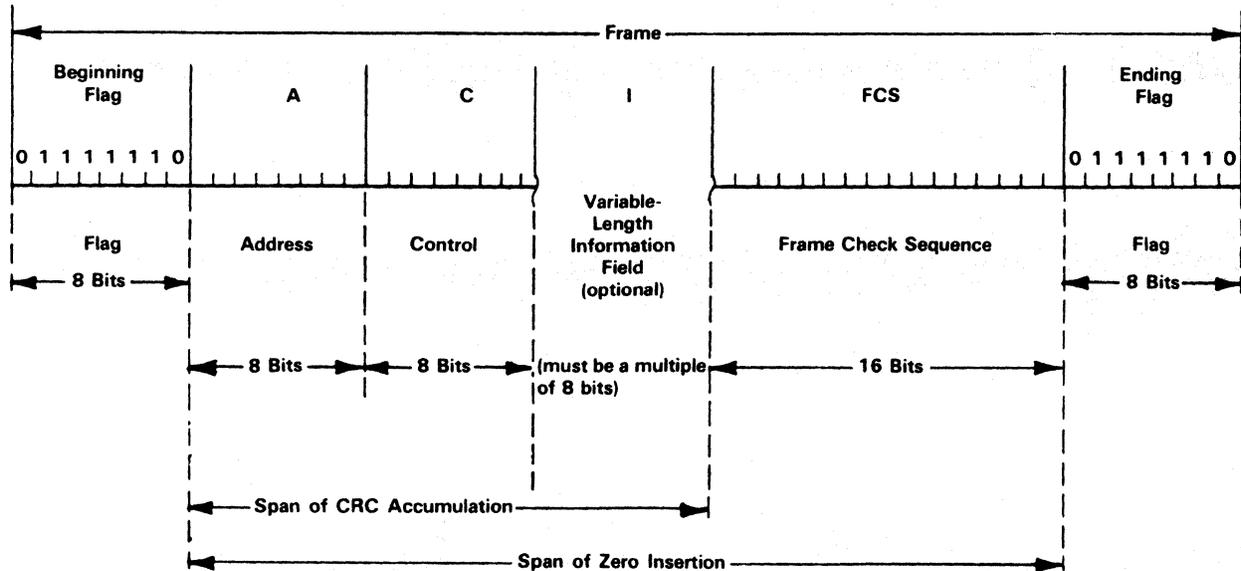
The transmission frame consists of Flag-Address-control-information-Frame Check Sequence-Flag. Each field has either eight bits or a multiple of eight bits.
