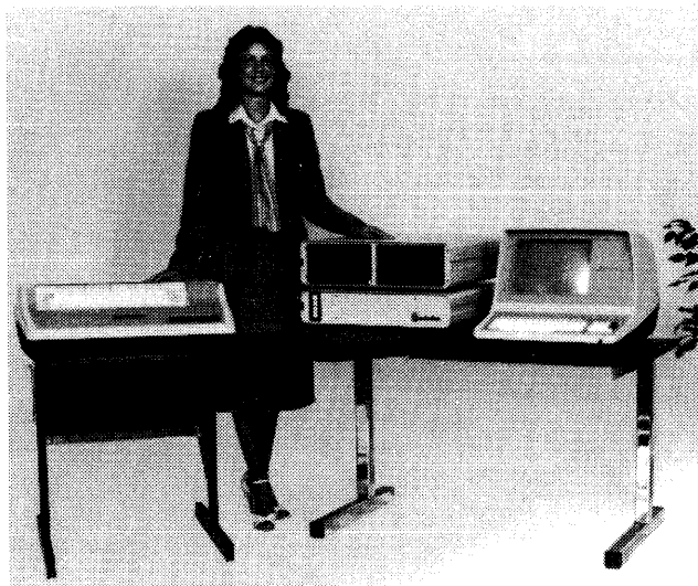
This MicroPlus features a 64K-byte CPU, a four-port multiplexer, two 1.2-megabyte dual-sided, double-density floppy disk drives, one CRT, and a 150-cps printer. The purchase price of the system as shown is $13,133.
