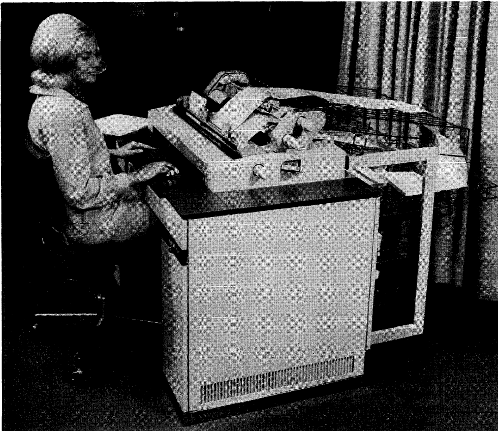
The Olivetti Auditronic 770 stores both programs and data on magnetic tape cartridges. The basic cartridge holds up to 36,960 characters, and an optional "supplementary memory" stores an additional 57,750 characters. An internal data memory holds 841 characters. Forms-handling facilities are unusually flexible.
