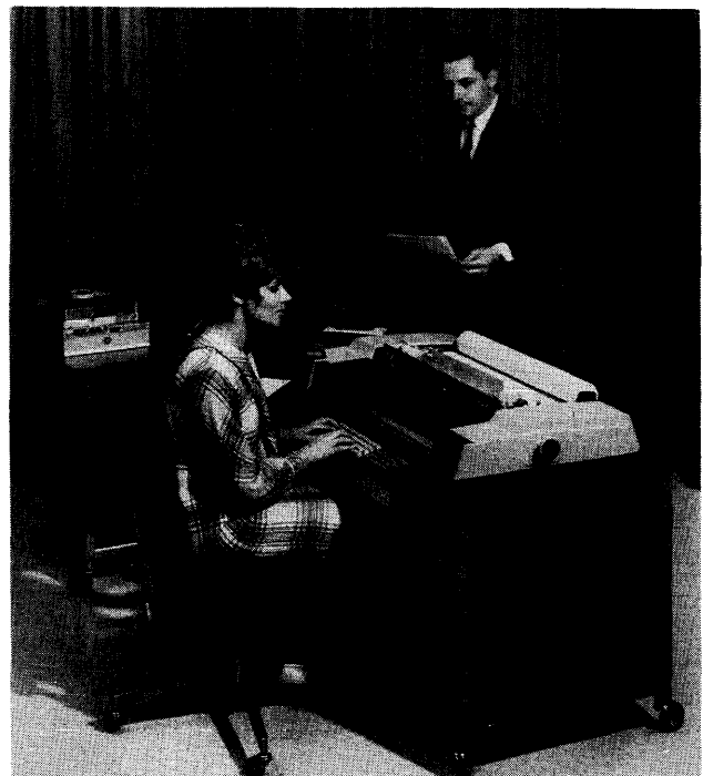
The Burroughs L 4000, like the other models of Burroughs' popular L Series accounting computers and TC Series communications terminals, features a magnetic disc memory that holds data, the user's programs, and "firmware" (microprogramming) which controls the system's arithmetic and logic operations. The 20-char/sec "ball printer" uses a print sphere similar to the IBM Selectric print element.
