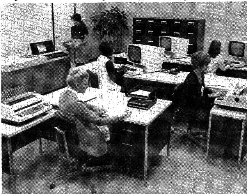
*This typical 3790 system installation demonstrates the operating flexibility that can be derived by mixing 3277 Display Stations and 3793 Keyboard-Printers to serve various business applications. The 3791 Controller with line printer is shown at left.*
