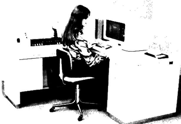
*The System/34 workstation utilizes a 5251-11 CRT Display Station, with its 4600 Keyboard, and a 5256 Printer.*
