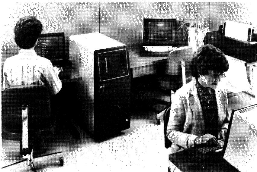
The Model 585 includes a new processor with integral Winchester-type disk storage for program loading and storage. The system supports up to 512K bytes of main memory, up to 342 megabytes of disk storage (internal plus external drives), and up to 16 CRT terminals and printers in any combination.
