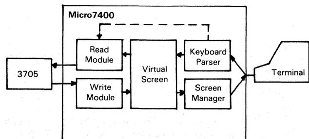
➤ Figure 1. Micro7400 functional block diagram.
