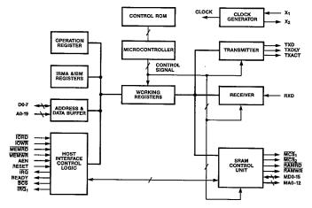
Figure 1. 82C570 Functional Block Diagram
