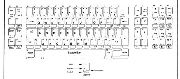
Figure F-1: Attribute Select Typewriter/APL Keyboard with Position Numbers
