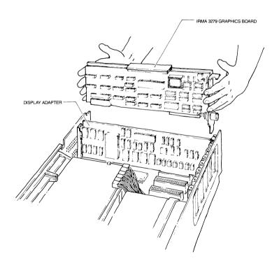
STEP 10: Secure the board with the screw you removed in step 10.
