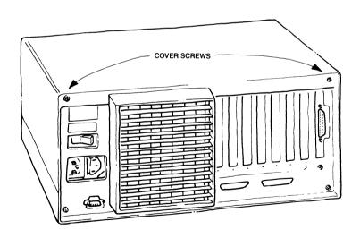
STEP 7: Carefully slide the cover forward about half an inch, then lift it up and remove it as shown in the following diagram.
