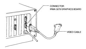
STEP 16: Connect the male end of the video cable to the female socket on the CGA or EGA card.
