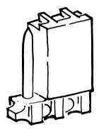
Figure 1-3: J1 Jumper Setting for Non-EGAs
