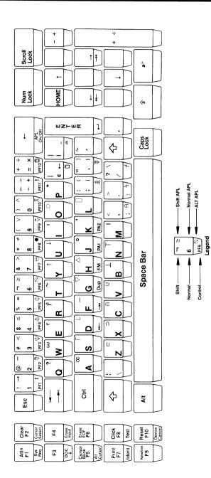
Figure A-3: APL Typewriter Keyboard
