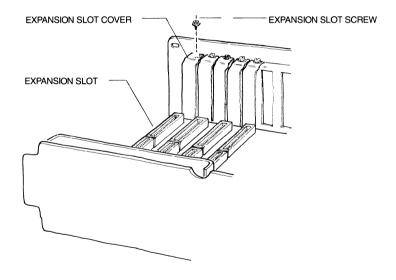
STEP 8: If you are using the IBM PC or PC XT, insert the plastic card guide into the holes that correspond to the expansion slot where you will install IRMA 3279 Graphics (or the display adapter if a card guide is already in the IRMA 3279 Graphics slot).
