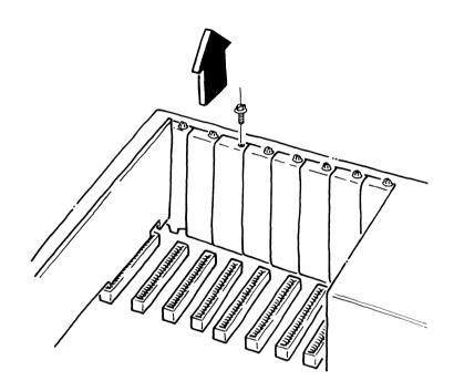
STEP 10: Insert the IRMA 3279 Graphics board into the expansion slot with the sockets of the board projecting out of the back of the system unit.
