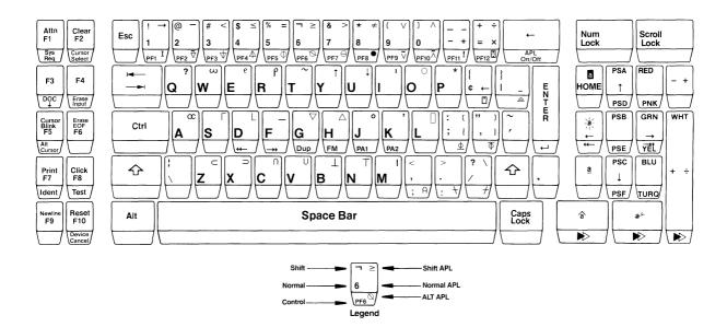
Figure A-1: Attribute Select Typewriter/APL Keyboard (default keyboard)
