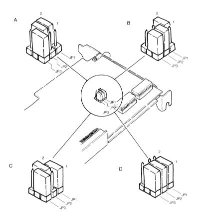
Figure 1-4: Base Address Jumper Settings
