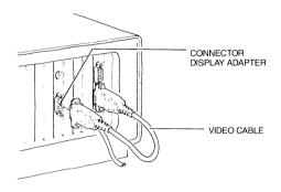
STEP 17: Connect the male end of the cable from your display unit to the female socket at the top of the emulator board.
