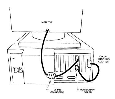
STEP 16: Reconnect all cables, including the power cord, plug the necessary cords into electrical outlets, and boot your computer with DOS.
