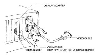
STEP 18: Connect the male end of the video cable to the female socket on the CGA or EGA.
