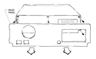
STEP 6: Carefully slide the cover forward and remove it.
