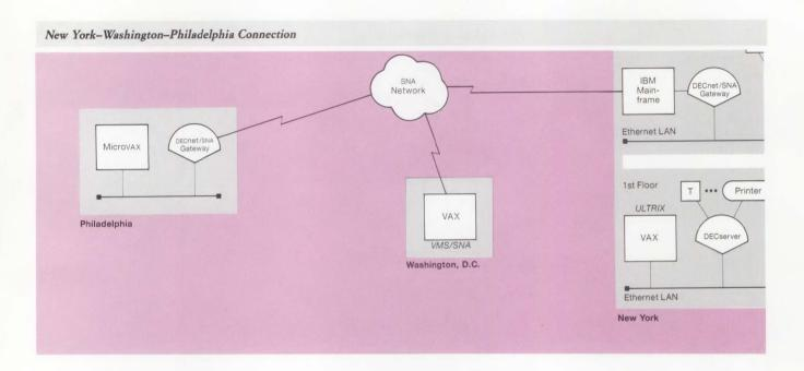
When volume and throughput warrants, Baker Company can upgrade the DECnet/SNA communications link on the second floor of the New York building to a DECnet/SNA Gateway for Channel Transport to handle more users and more sessions at higher throughput. A Refer to Section 4 for information on DECnet/SNA capabilities.
