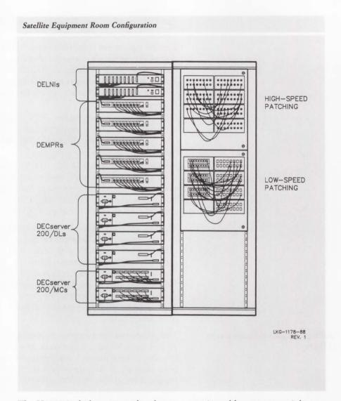
The H3120 includes two steel racks, power strip, cable managers, eight sets of rackmount brackets for DECservers or DEMPRs, one set of rackmount brackets for the DELNI, and two patch frame panels for mounting cable patch panels. Customers select patch panels, patch cords, and other accessories from the menu of building block kits to meet their application needs. ▲ Refer to "Cabinet Building Block Kits" in this section for more information.
