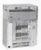
The DECserver 550 terminal server is a terminal switch capable of connecting large concentrations of VT and/or IBM 3270 CUT terminals, serial printers, and modems to one or many hosts on an 802.3/Ethernet local area network. It can also be used to connect other vendors' processors to the local area network, allowing access to terminal-server users. It is the high-end companion to the DECserver 200 terminal server.
