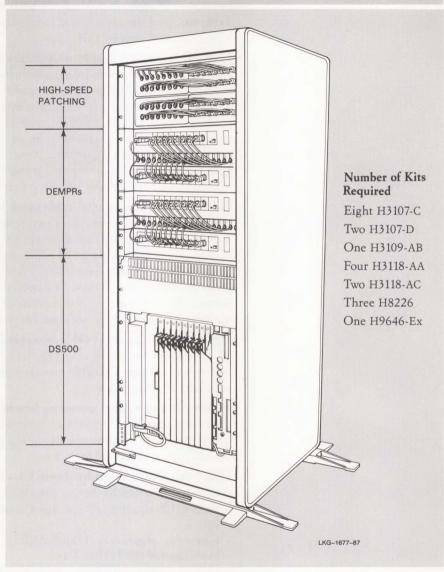
H9646-E Cabinet Configuration for 128 Low-speed, 32 High-speed Connections with No Patching
