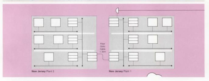
The fiber optic link provides Baker Company's research department with an environment impervious to lightning and electrical interference. Also, fiber optic cable is very difficult to tap into, it provides a secure environment—something that is very critical to the research department.
