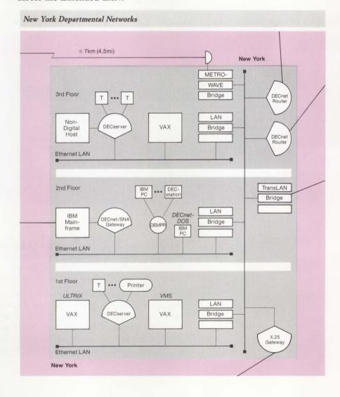
The filtering of data traffic allows Baker Company to have very high network performance on each floor and within each departmental LAN. The company retains the high performance of a single LAN without impacting the other LANs on the backbone. Remote Bridge Management Software (RBMS) simplifies the configuration and fault management of this extended LAN.
