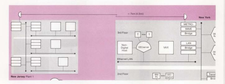
The METROWAVE Bridge provides a microwave connection in an Extended LAN environment, using the LAN Bridge 100 to deliver the same high performance, filtering capability, and reliability as other LAN Bridge products. ▲ Refer to "METROWAVE Bridge," Section 2.
