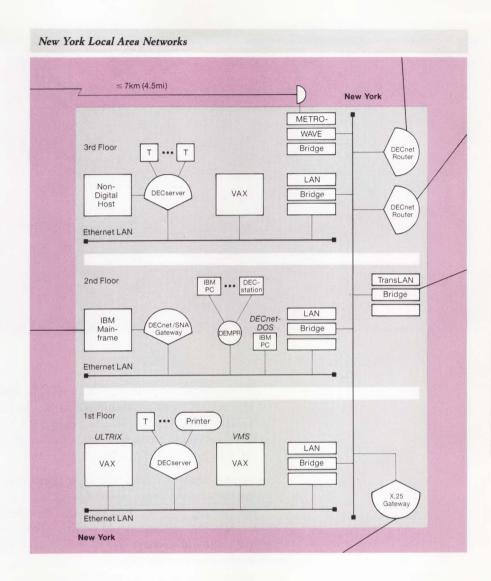
Baker Company has optimized its IBM/Digital connection by using its Digital desktop workstations to run application programs that reside on the IBM host, and by taking advantage of DECnet/SNA transport services.
