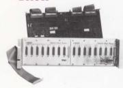
The DHU11 is a 16-line asynchronous communications controller with direct memory access (DMA) that provides local and remote connection between UNIBUS PDP-11 or VAX systems and EIA-232-C/CCITT V.28 or EIA-423-A/CCITT V.10 terminals, modems, serial printers, and data switches. The DHU11 supports operating speeds up to 38.4 Kb/s. Actual communications speed and throughput is dependent on current Digital operating systems and system configuration. Full modem control is available on all 16 lines.
