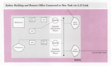
The Ethernet LAN in the Sydney building communicates with New York headquarters via an X.25 Gateway (X25 router 2000) connected through the Packet Switched Data Network (PSDN). The X25 router 2000 provides the optimum bandwidth-efficient solution with high-speed data communications based on the required data flow and volume.
