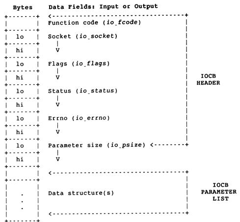
Figure 6-3: An IOCB Data Structure
