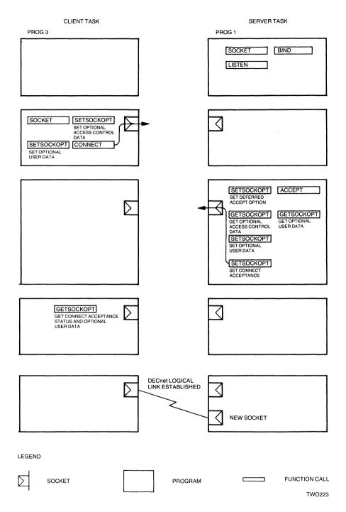
Figure 1-4: Establishing a DECnet Logical Link
