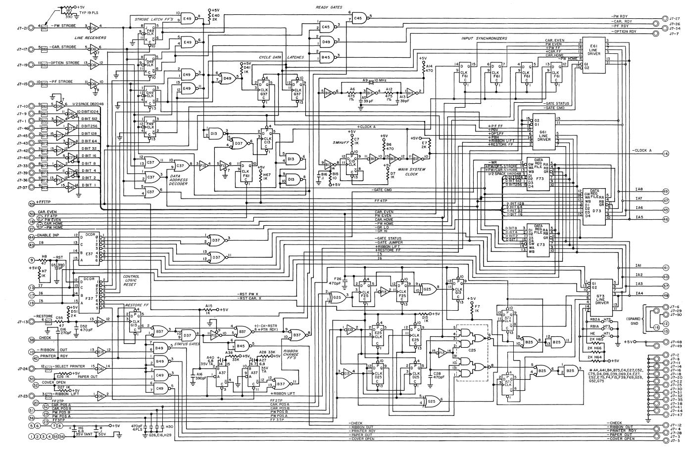
Figure 7-2a Logic #1 PCB Assy, Standard #40505-09 Rev B
