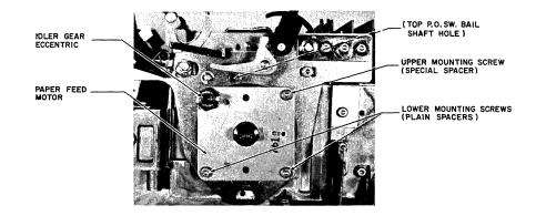
Figure 5-9 PAPER FEED MOTOR REMOVAL
