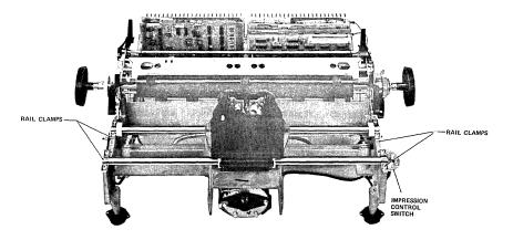
Figure 5-18 CARRIAGE RAIL CLAMPS
