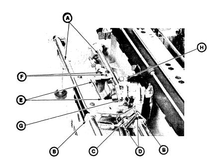
Figure 5-1 CARRIAGE SYSTEM LUBRICATION POINTS
