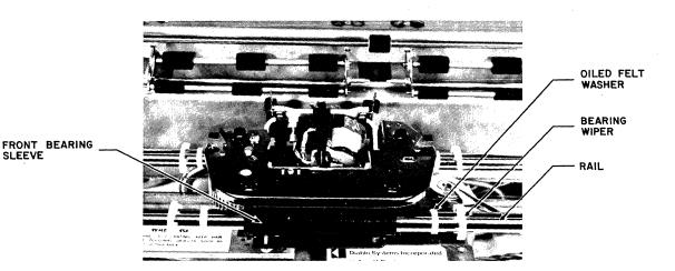
Figure 5-19 CARRIAGE AND RAIL REASSEMBLY
