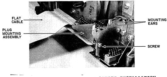
Figure 5-53 ADAPTER CABLE OPTION INSTALLATION
