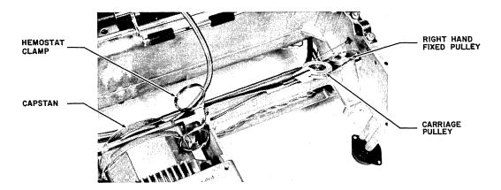
Figure 5-36 RIGHT-HAND CARRIAGE DRIVE CABLE INSTALLATION
