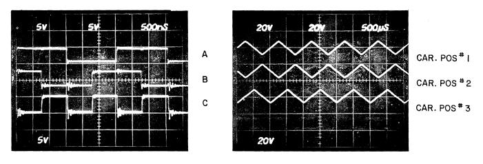
Figure 4-13 SERVO FEEDBACK DEMODULATOR/INTEGRATOR/AMPLIFIER WAVEFORMS
