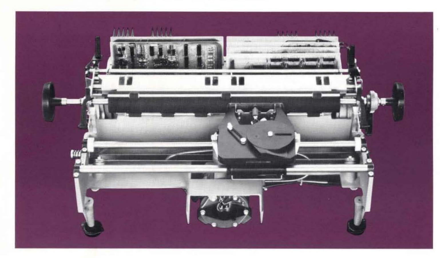
The Diablo HyType<sup>®</sup> II 1355 WP with the metal print wheel is designed specifically for OEM word processing applications.
