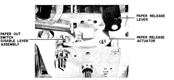
Figure 5-48 TOP PAPER OUT SWITCH DISABLE ASSEMBLY
