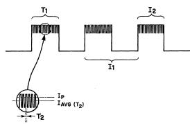
$\begin{array}{rcl} I_1 &=& 4.5 \mbox{ Amps Average} \\ I_2 &=& 9 \mbox{ Amps } @ \mbox{ 40\% Duty Cycle} \\ T_1 &=& 70 \mbox{ milliseconds maximum} \\ I_p &=& 14 \mbox{ Amps } @ \mbox{ 40\% Duty Cycle} \\ T_2 &=& 30 \mbox{ microseconds} \end{array}$
