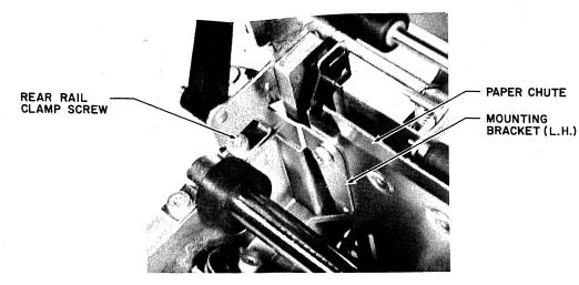
Figure 5-42 UPPER PAPER CHUTE MOUNTING BRACKET INSTALLATION
