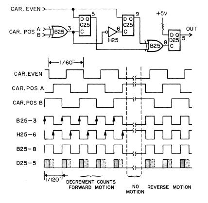
Figure 4-5 CARRIAGE DIFFERENCE COUNTER DECREMENT DRIVE
