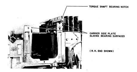
Figure 5-10 CARRIER SYSTEMS REPLACEMENT
