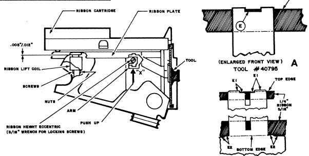
Figure 5-23 RIBBON HEIGHT ADJUSTMENT
