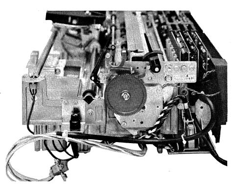
Figure 5-60 AC AND DC CABLE INSTALLATION
