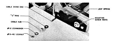
Figure 5-37 CARRIAGE DRIVE CABLE TENSION SPRING ASSEMBLY
