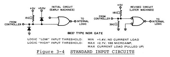
The input of the printer line receiver must be <u>pulled up</u> to the HI logic state. For this reason it cannot be driven by an open collector driver without collector resistance. The collector resistance inside the printer is 150 Ohms. The circuits are configured as shown in Figure 3-4.
