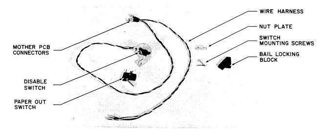
Figure 5-43 BOTTOM FEED PAPER CHUTE PAPER OUT SWITCH PARTS
