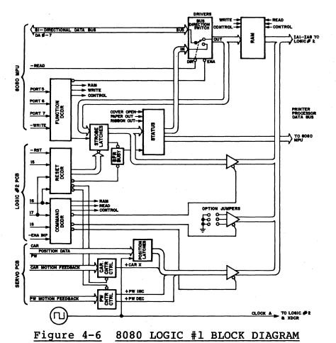
Refer to Figure 4-6. The transfer of a printer command from the 8080 MPU to the Logic #2 microprocessor involves the following steps:
