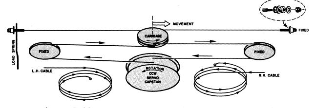
Figure 5-35 CARRIAGE CABLE DRIVE SYSTEM SCHEMATIC
