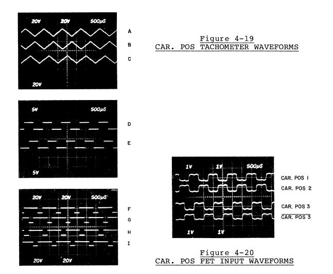
Figure 4-19 shows waveforms taken in these circuits.
