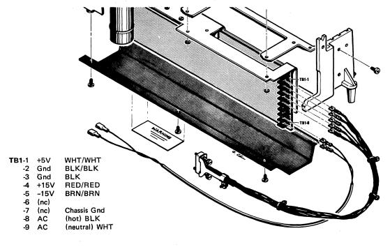
Figure 5-59 AC AND DC POWER CONNECTIONS
