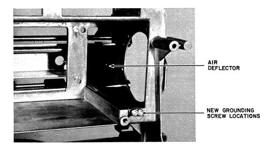
Figure 5-55 FAN AIR DEFLECTOR INSTALLATION
