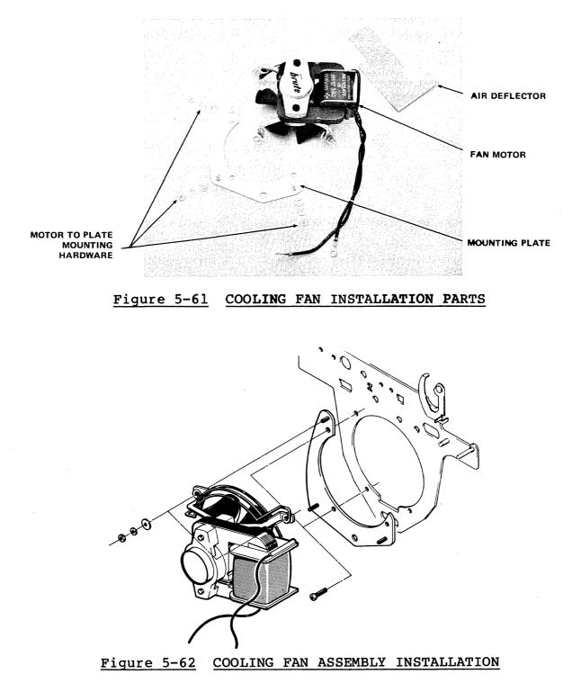
1. Assemble and identify the various parts needed for installation of the cooling fan, as shown in Figure 5-61.
