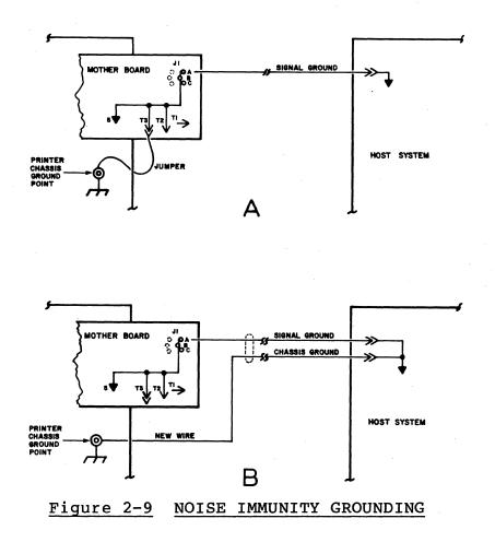
tie printer chassis ground to source chassis ground. In addition, care should be taken to strap any cover halves together, and to the printer chassis ground.
