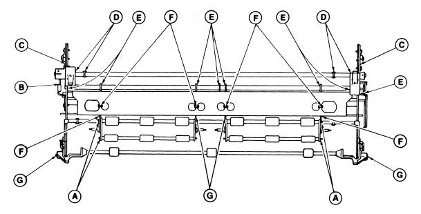
Figure 5-3 CARRIER SYSTEM LUBRICATION POINTS
