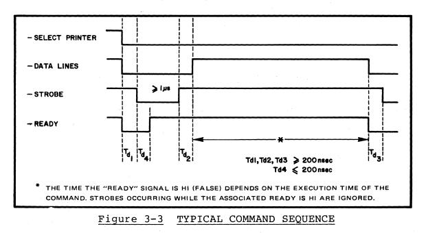
The HyType II Printer will accept data to select a character, move the carriage, or feed paper only when the corresponding STROBE pulse is present on the interface. The timing diagram in Figure 3-3 il-
