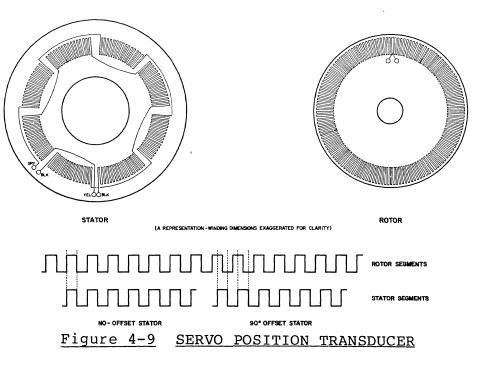
As shown in Figure 4-9, the stator has an eight segment winding, with alternate segments connected together to form two groups of four segments each. The four segments of one group are displaced laterally from the other group by a distance equal to one-half a winding width. This displacement is equal to a  $90^{\circ}$  phase difference.
