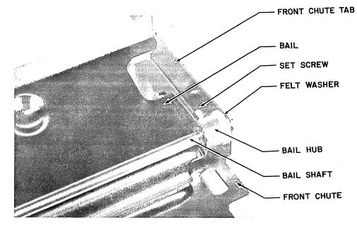
Figure 5-40 BAIL AND FRONT CHUTE ASSEMBLY
