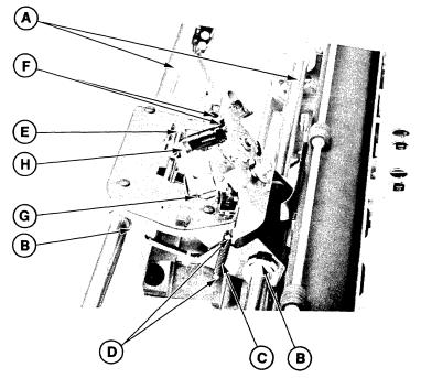
Figure 5-2 CARRIAGE SYSTEM LUBRICATION POINTS
