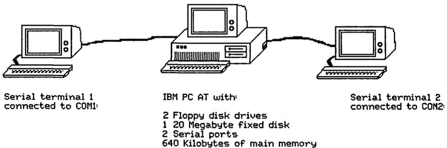
**Figure 3.8** The IBM PC AT can be used as a multiuser system under Concurrent PC DOS. The two serial ports, COM1: and COM2:, can be configured as additional consoles.
