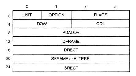
Figure 7-4. COPY/ALTER Parameter Block
