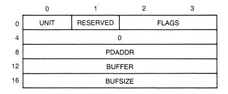
Figure 10-6. Printer Driver SET Parameter Block
