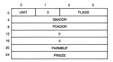
Figure 8–13. SPECIAL Function 3 Parameter Block
