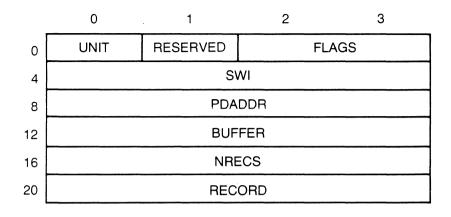
Figure 8-8. READ Parameter Block
