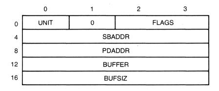
Figure 8-10. SPECIAL Function 0 Parameter Block
