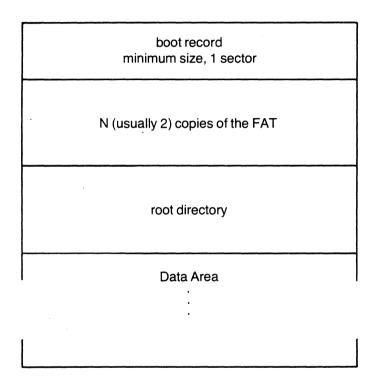
Figure 12-1. FlexOS Disk Layout
