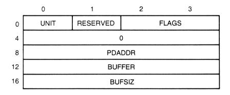
Figure 9-6. Port Driver SET Parameter Block
