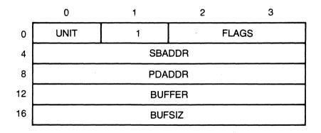
Figure 8–11. SPECIAL Function 1 Parameter Block
