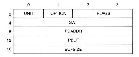
Figure 10–3. Printer Driver WRITE Parameter Block
