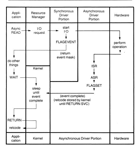
Figure 2-2. Asynchronous I/O Request
