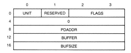
Figure 10-4. Printer Driver GET Parameter Block
