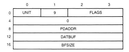
Figure 8-16. SPECIAL Function 9 Parameter Block
