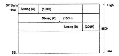
Figure 7-4. Combining Segments with Stack Combination
