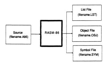
Figure 1-1. RASM-86 Source and Object Files
