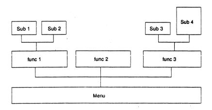
Figure 8-2. Tree Structure of Overlays
