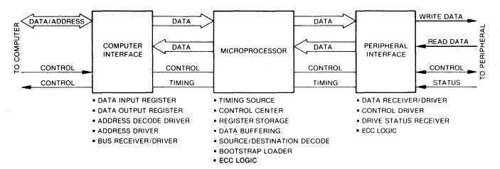
Figure 5-2. Simplified Block Diagram
