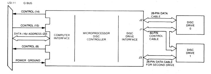
Figure 1-1. Disc Controller System Simplified Diagram
