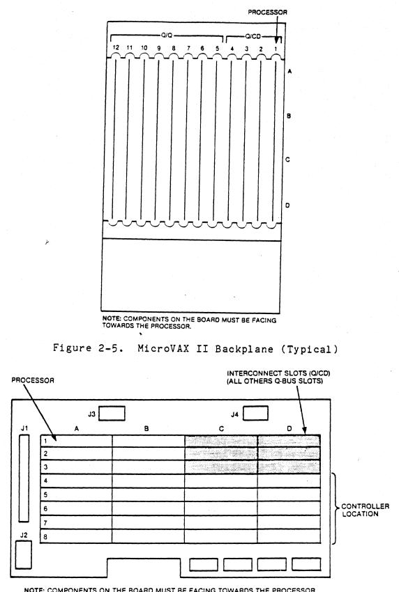
NOTE: COMPONENTS ON THE BOARD MUST BE FACING TOWARDS THE PROCESSOR.
