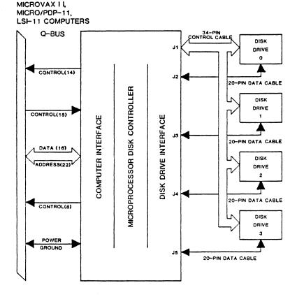
Figure 1-1. Disk System, Simplified
