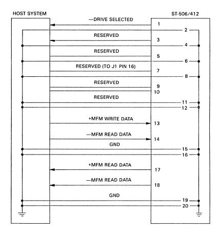
Figure 6-5. Data Pin/Signal Assignments at Disk Drive Interface
