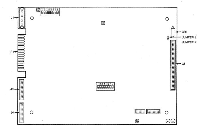
Figure 3-1. MD01 Switch and Jumper Locations
