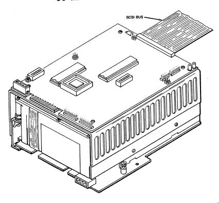
Figure 3-4. Connecting SCSI bus to MD01 Controller
