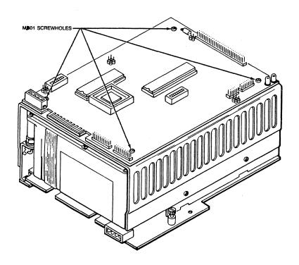
Figure 3-2. Installing MDO1 Controller on Mounting Bracket
