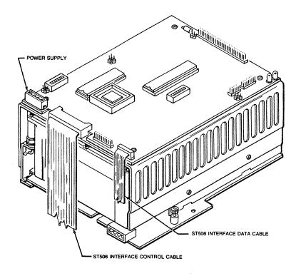
Figure 3-3. Connecting Disk Drive Data and Control Cables to MD01 Controller
