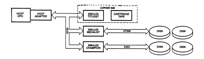
Figure 1-2. Sample SCSI Bus System Configuration
