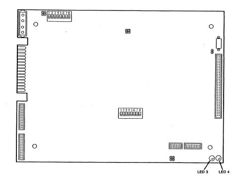
Figure 4-1. Location of LEDs on MD01 Controller
