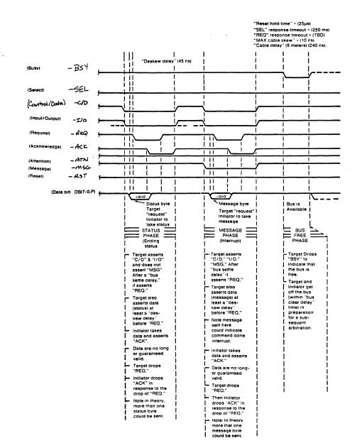
Figure 6-3. SCSI Bus Timing Diagram (Sheet 3 of 3)
