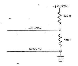
Figure 6-2. SCSI Bus Signals Termination
