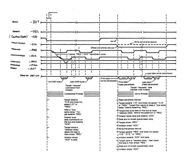
Figure 6-3. SCSI Bus Timing Diagram (Sheet 2 of 3)
