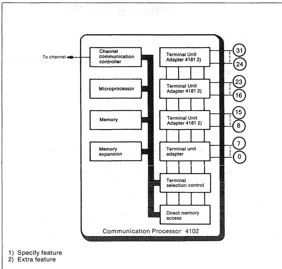
Fig. 5. Block diagram of Communication Processor 4102
