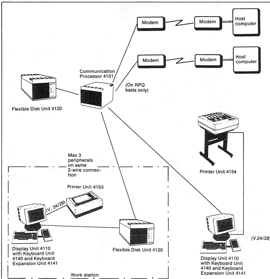
Fig. 1. Cluster configuration connected to remote host computers
