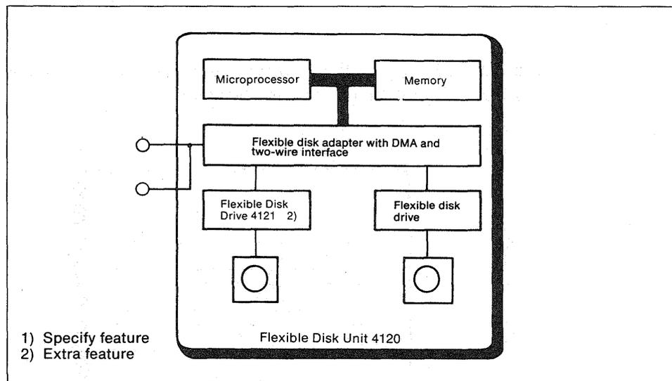
Fig. 15. Block diagram of Flexible Disk Unit 4120
