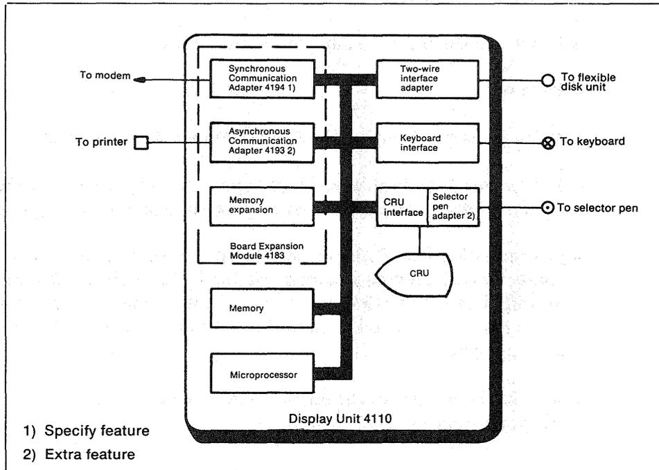
Fig. 9. Block diagram of Display Unit 4110 in single display-unit configuration
