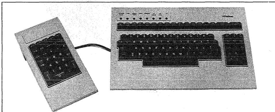
Fig. 10. Keyboard Unit 4140 with Keyboard Expansion Unit 4141
