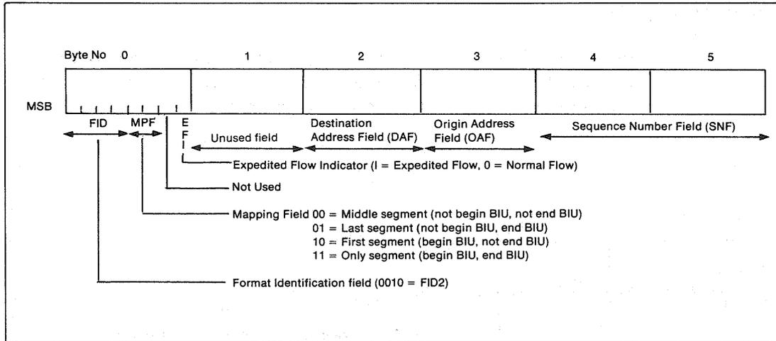
Fig. 6. Transmission header format
