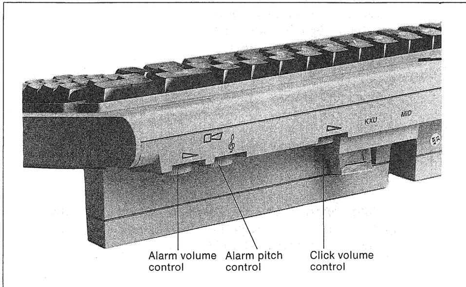
Fig. 4. Keyboard controls
