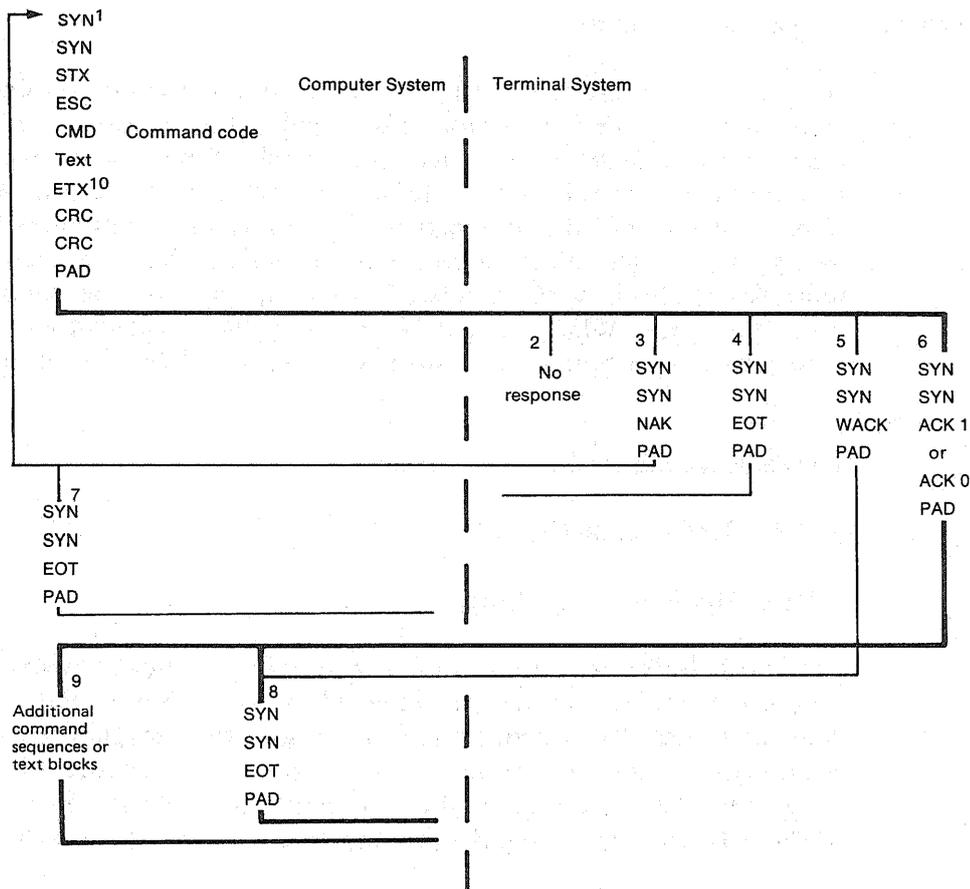
Fig. 3. Write-type and control commands, sequence diagram
