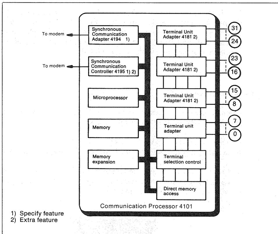
Fig. 3. Block diagram of Communication Processor 4101
