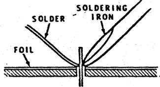
3. As the solder begins to melt, allow it to flow around the connection. Then remove the solder and the iron and let the connection cool.
