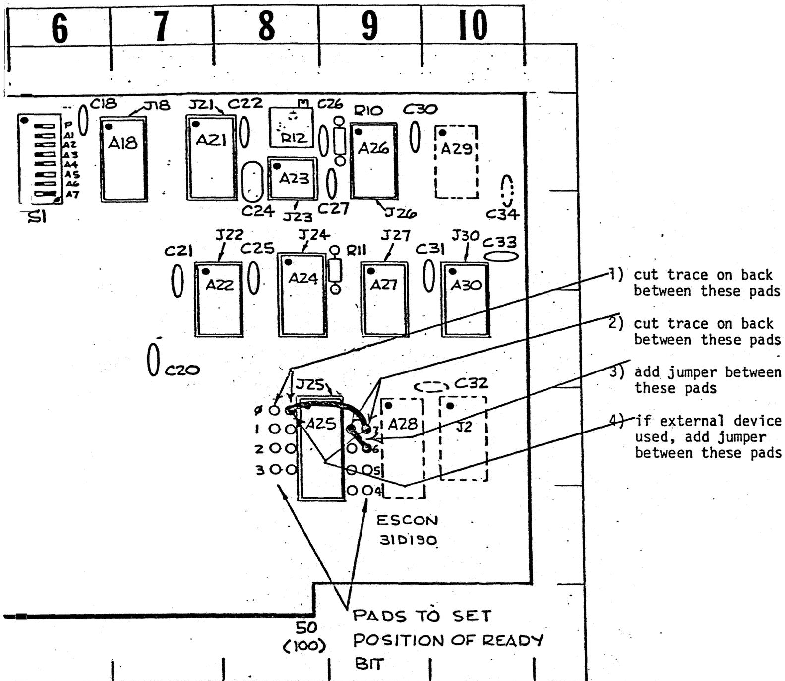
Figure 3. Changes Required to Adapt Interface Board to Correspond to the SIO port used in Altair Basic.
