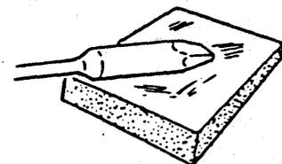
Use rosin core, radio-type solder (60:40 or 50:50 tin-lead content) for all soldering in the kit. The Warranty will be void and we will not service any kit in which acid core solder or paste fluxes have been used.
