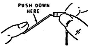
3. Push the leads through the holes at the proper location on the circuit board. The end with color bands may be positioned either way.
