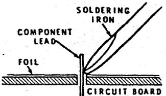
2. Then apply solder to the other side of the connection. **IMPORTANT:** Let the heated lead and the circuit board foil melt the solder.
