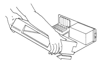
Figure 3-2 Removing the Cover
