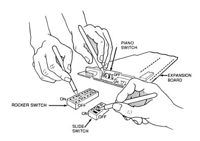
Figure 3-27. Setting Slide and Rocker Switches
