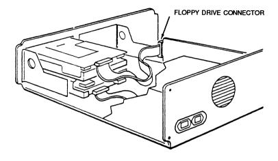
Figure 3-24. Connecting the Floppy Controller
