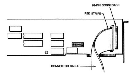
Figure 3-4 Connecting the Ribbon Cable
