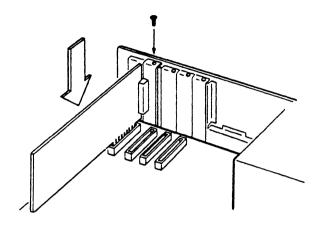
Figure 3-13 Installing the Tape Controller Card
