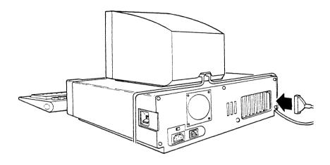
Figure 3-14 Connecting the Shielded Round Cable to the Tape Controller Card
