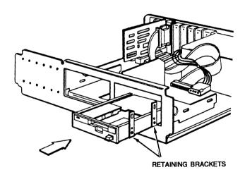
Figure 3-8 Connecting Retaining Brackets to an Internal Tape Drive
