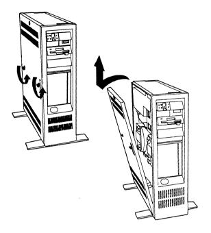
Figure 3-20 Loosening the Model 60 Cover Mounting Screws
