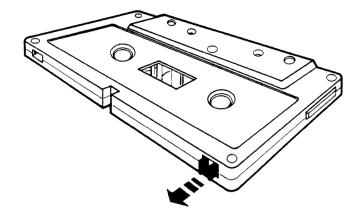
**Figure 3-26.** Write Enabling/Protecting a Cassette Tape
