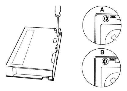
**Figure 3-25.** Write Enabling/Protecting a Cartridge Tape
