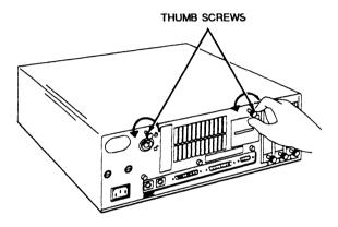
Figure 3-16 Model 50 Cover Mounting Thumb Screws
