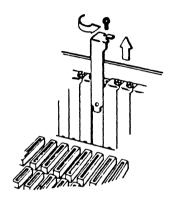
Figure 3-12 Removing a Slot Cover
