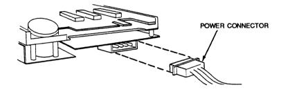
Figure 3-7 Applying Power to the Tape Drive
