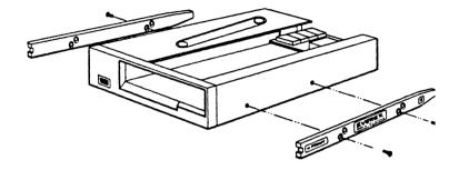
Figure 3-9 Attaching AT Slide Rails to an Internal Tape Drive
