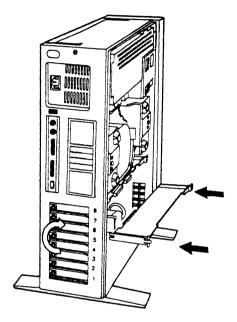
Figure 3-22 Installing the Tape Controller Card in the Model 60
