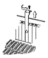
Figure 3-3 Removing a Slot Cover
