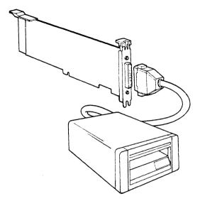
**Figure 3-23** Cabling the Tape Drive and Controller Card
