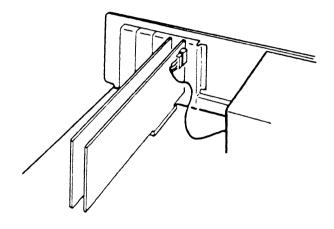
Figure 3-15 Applying Power to the Tape Controller
