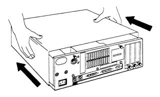
Figure 3-17 Removing the Cover of the Model 50
