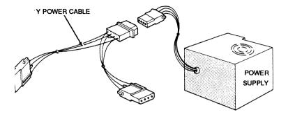
Figure 1 Adding a Y Power Cable
