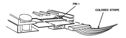
Figure 3-6 Connecting the Ribbon Cable to the Tape Drive
