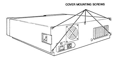
Figure 3-10 Cover Mounting Screws
