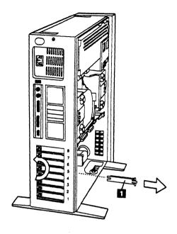
Figure 3-21 Removing a Slot Cover from the Model 60
