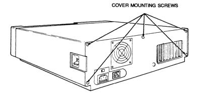
Figure 3-1 Cover Mounting Screws
