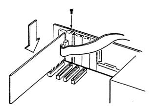
Figure 3-5 Installing the Tape Controller Card
