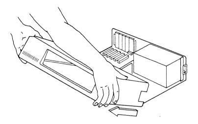
Figure 3-11 Removing the Cover
