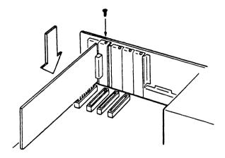
Figure 3-13 Installing the Tape Controller Card
