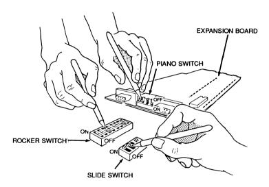
Figure 3-26. Setting Slide and Rocker Switches
