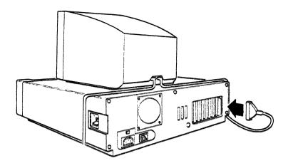
Figure 3-14 Connecting the Shielded Round Cable to the Tape Controller Card
