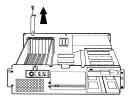
Figure 3-12 Removing a Slot Cover
