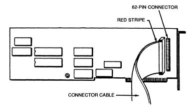
Figure 3-4 Connecting the Ribbon Cable
