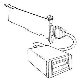
Figure 3-23 Cabling the Tape Drive and Controller Card
