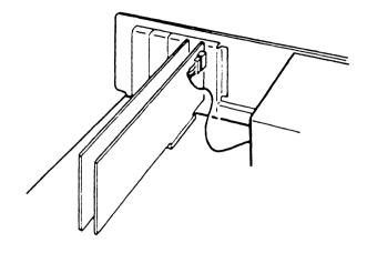
Figure 3-15 Applying Power to the Tape Controller
