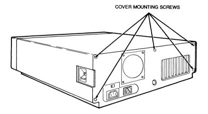
Figure 3-10 Cover Mounting Screws
