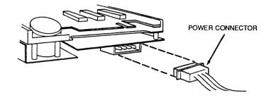
Figure 3-7 Applying Power to the Tape Drive
