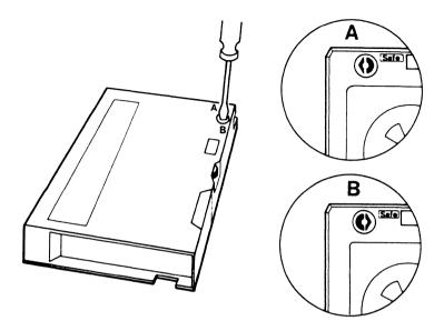
**Figure 3-24.** Write Enabling/Protecting a Cartridge Tape
