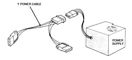
Figure 2-1 Adding a Y Power Cable
