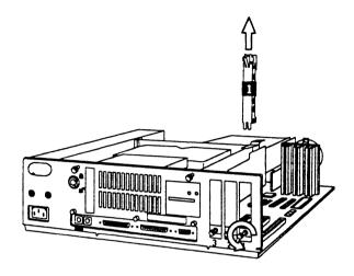
**Figure 3-18** Removing a Slot Cover from the Model 50
