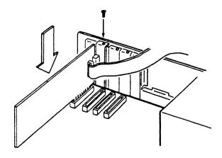
Figure 3-5 Installing the Tape Controller Card
