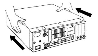
Figure 3-17 Removing the Cover of the Model 50
