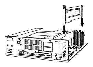
Figure 3-19 Installing the Tape Controller Card in the Model 50
