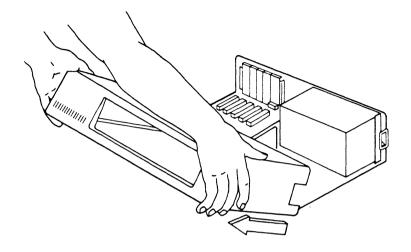
Figure 3-11 Removing the Cover
