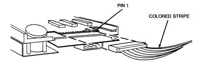
Figure 3-6 Connecting the Ribbon Cable to the Tape Drive
