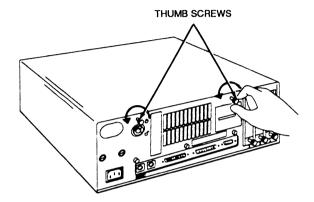
Figure 3-16 Model 50 Cover Mounting Thumb Screws
