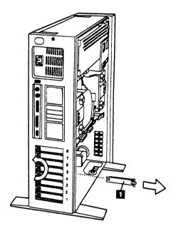
**Figure 3-21** Removing a Slot Cover from the Model 60
