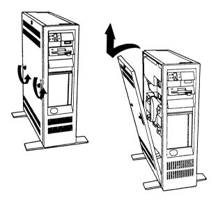
Figure 3-20 Loosening the Model 60 Cover Mounting Screws
