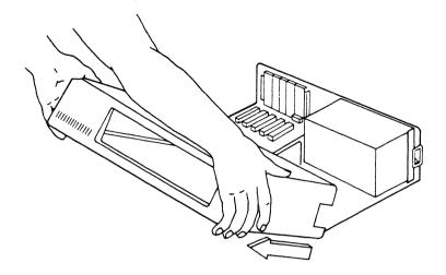
Figure 3-2 Removing the Cover
