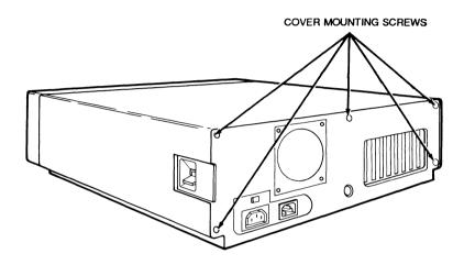
Figure 3-1 Cover Mounting Screws
