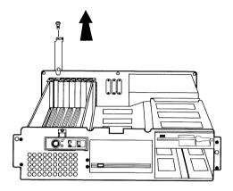
Figure 3-3 Removing a Slot Cover
