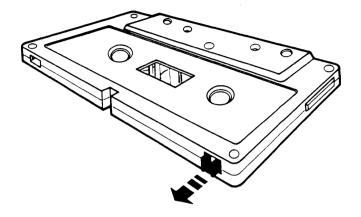
**Figure 3-25.** Write Enabling/Protecting a Cassette Tape
