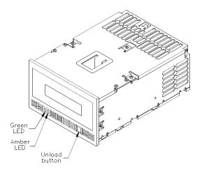
Figure 8 Unload button and LEDs
