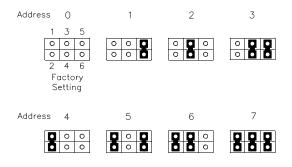
Figure 2 Jumper settings for the SCSI ID
