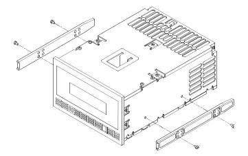
Figure 5 Attaching the slide rails to the tape drive
