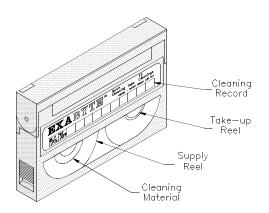
Figure 10 Exabyte 8mm Cleaning Cartridge with label showing cleaning cycles left
