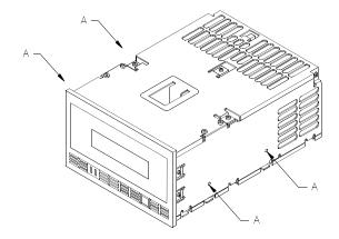
Figure 14 Mounting holes on the sides of the tape drive
