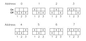
Figure 13 DIP switch settings for the SCSI ID
