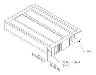
Figure 9 Write-protect switch on an EXATAPE 8mm data cartridge
