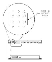
Figure 1 SCSI ID jumper block
