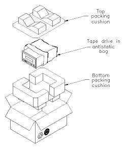
Figure 12 Single-pack carton and packing materials
