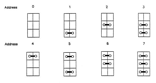
Figure 9-6 SCSI ID Jumper Connections for the DS3 Card
