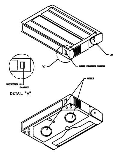
Figure 10-2 8mm Data Cartridge
