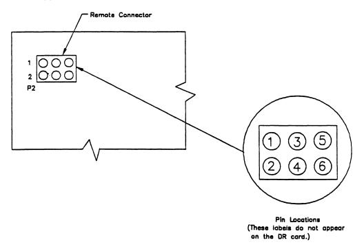
Figure 9-2 Remote Connector on the DR Card
