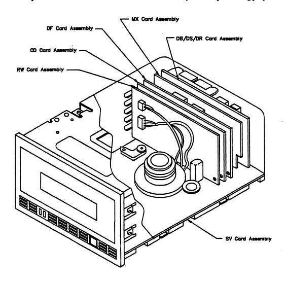
Figure 2-1 EXB-8200 Cartridge Tape Subsystem
