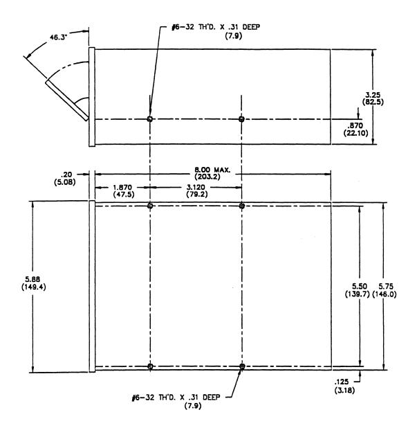
Figure 9-7 EXB-8200 Envelope and Mounting Hole Dimensions in Inches (and Millimeters)
