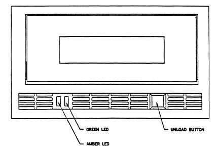
Figure 10-1 EXB-8200 Front Panel Controls and Indicators
