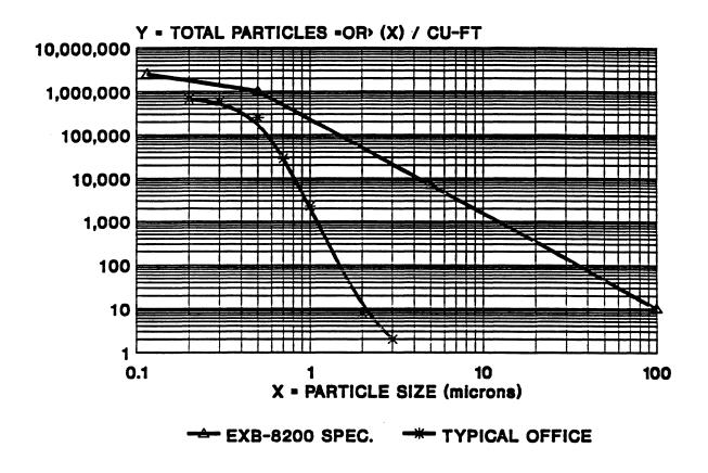
Figure 7-2 EXB-8200 Particulate Contamination Specification vs. Typical Office
