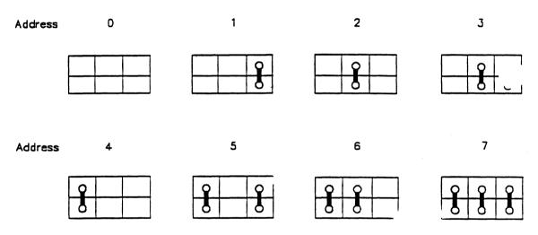
Figure 9-3 SCSI ID Jumper Connections for the DR Card
