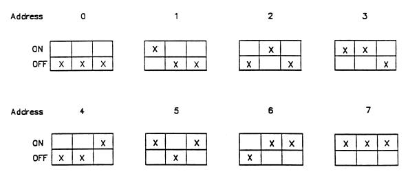
Figure 9-5 SCSI ID DIP Switch Settings for the DS3 and DB Cards Figure 9-6 shows the jumper connections and the corresponding SCSI IDs for the DS3 card.
