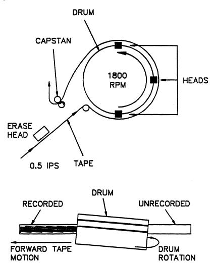
Figure 2-2 EXB-8200 Helical Scan Recording
