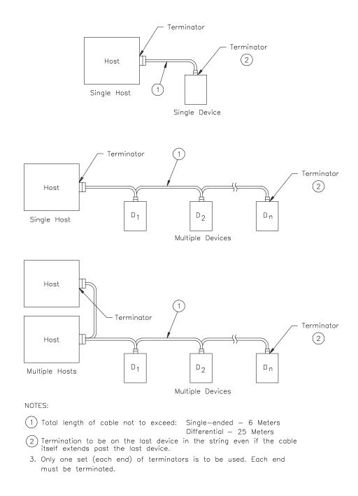
Figure 2-1 Typical Configurations for Single-Ended and Differential Cable
