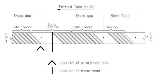
Figure 24-7 Physical Position after a Backward Space Filemark Operation
