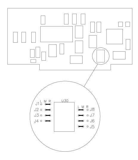
Figure A-1 Jumper Locations on the Level 1 MX Card
