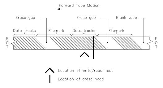
Figure 24-5 Physical Position after a Forward Space Filemark Operation Ending before Additional Data
