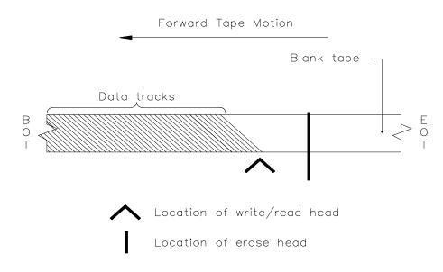
Figure 24-8 Physical Position after a Write Operation
