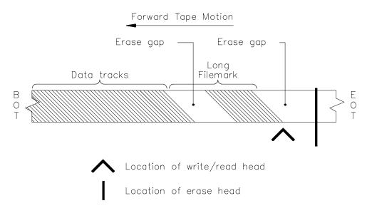
Figure 24-4 Physical Position after a Forward Space Filemark Operation Ending at the End of Data
