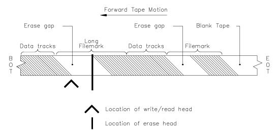
Figure 24-1 Physical Position after a Read Operation Ending Before a Long File-
