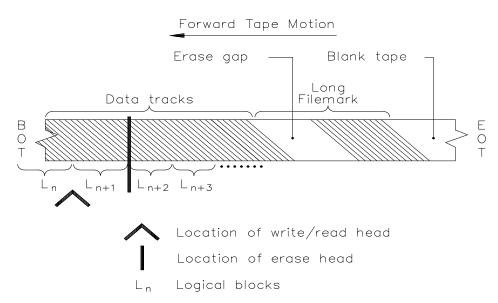
Figure 24-3 Physical Position after a Forward Space Block Operation
