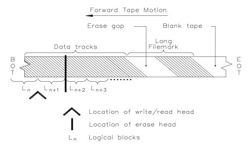
Figure 24-2 Physical Position after a Read Operation Ending in Data
