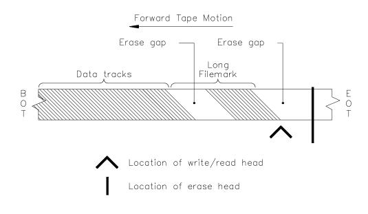
Figure 24-9 Physical Position after a Write Filemarks Operation
