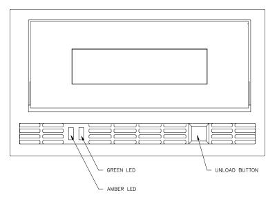
Figure 23-1 Unload Button on the EXB-8200's Front Panel
