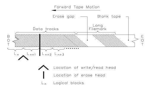
Figure 24-6 Physical Position after a Backward Space Block Operation
